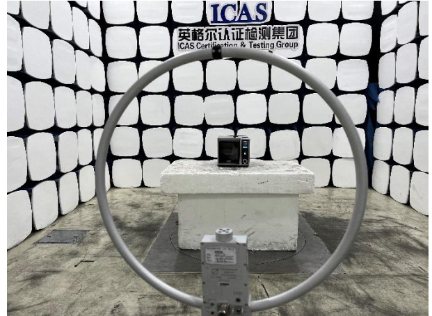
Radiated Emission Test Set-up for Below 30MHz
