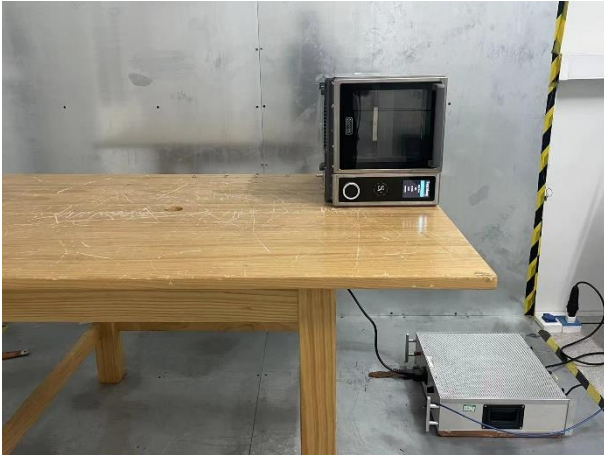
Radiated Emission Test Set-up for 30M-1GHz
