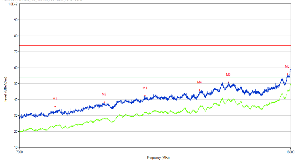
REmission Test case_FCC_Part 15C_FCC 15.247_7GHz-18GHz
