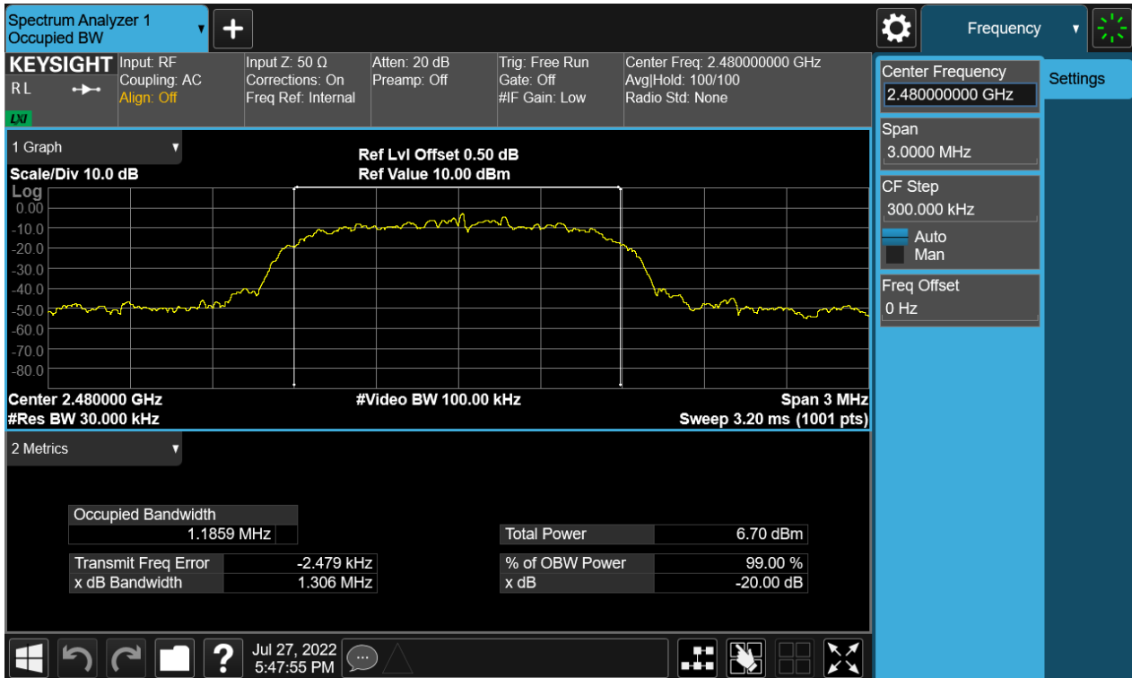
Figure 18: 20dB Bandwidth, 2480MHz, 8-DPSK
