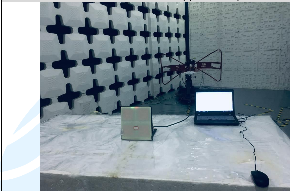
Radiated emission Test Setup (30 MHz~1 GHz)
