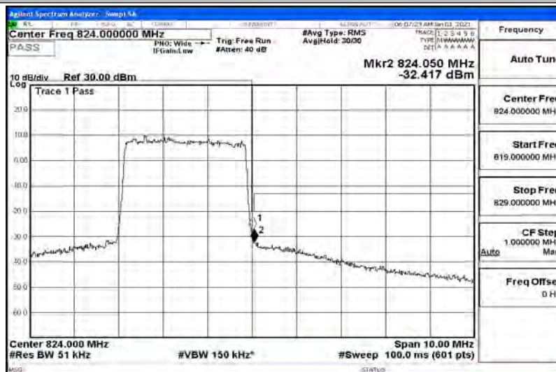
Band Edge Test Graph(s) (Channel Bandwidth: 3 MHz)_HCH_16QAM
