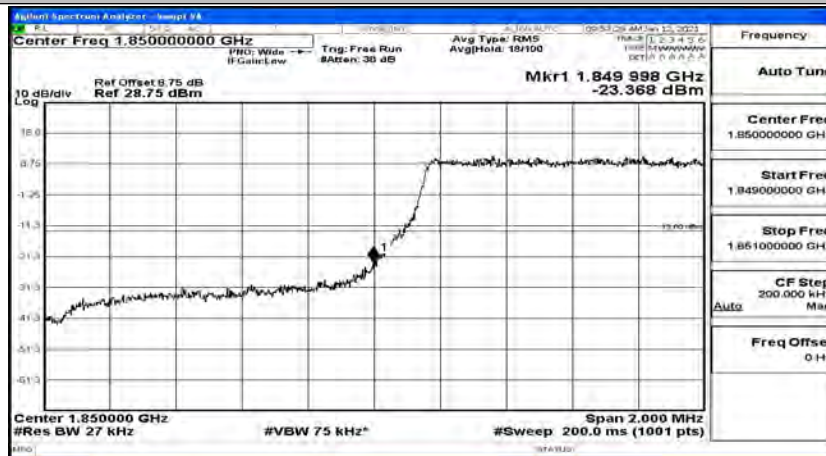
Band Edge Test Graph(s) (Channel Bandwidth: 1.4 MHz)_LCH_QPSK
