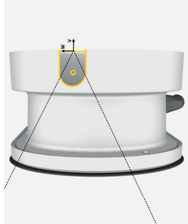
Fig. 12: Centering to position the holesaw
