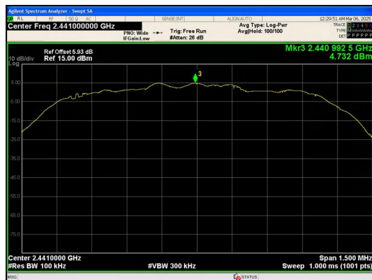
In-Band Reference Level 8DPSK_3-DH1_Channel 39
