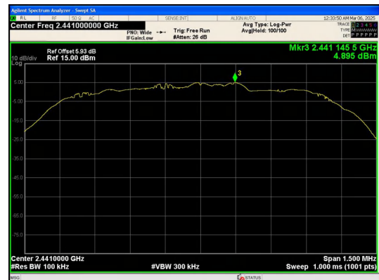
In-Band Reference Level 8DPSK_3-DH5_Channel 39
