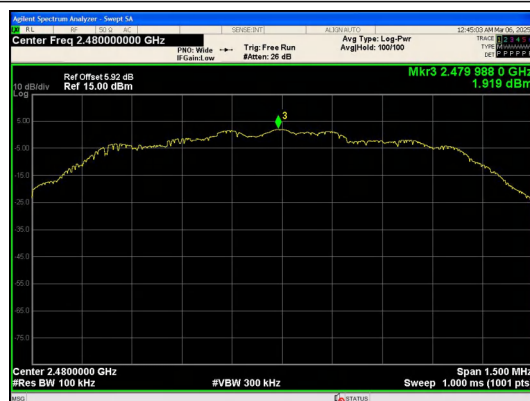
In-Band Reference Level 8DPSK_3-DH3_Channel 78
