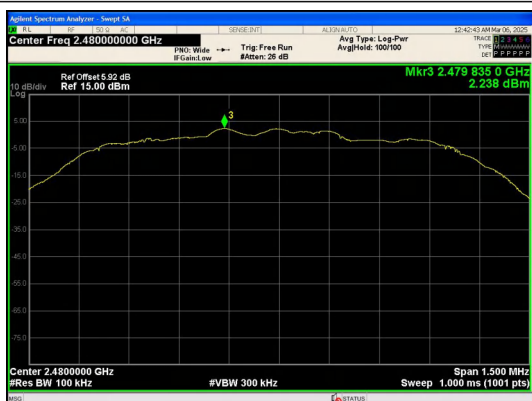
In-Band Reference Level 8DPSK_3-DH1_Channel 78
