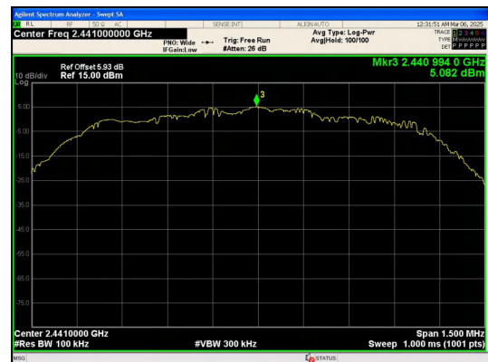
In-Band Reference Level 8DPSK_3-DH3_Channel 39
