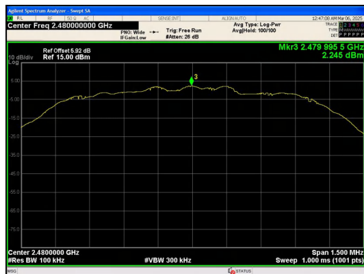
In-Band Reference Level 8DPSK_3-DH5_Channel 78
