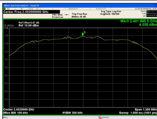
In-Band Reference Level 8DPSK_3-DH5_Channel 0
