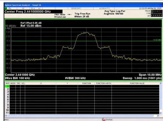
Out Of Band Emission 8DPSK_3-DH3_Channel 39
