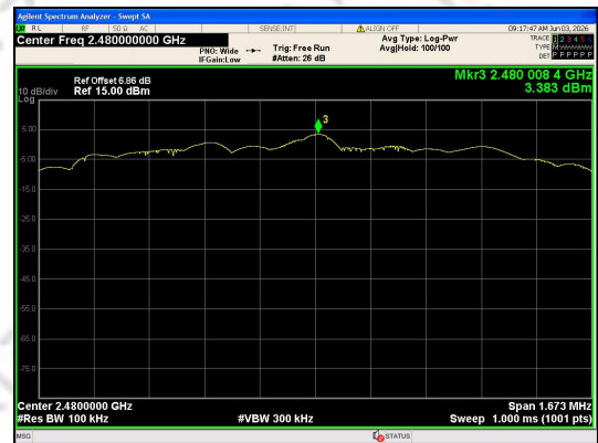
In-Band Reference Level BLE 2M_Channel 39
