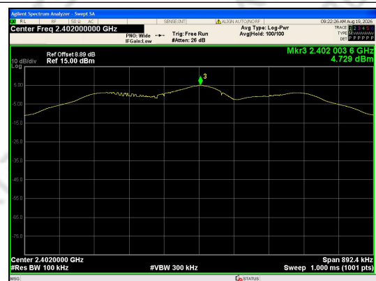
In-Band Reference Level LE Coded (S=8)_Channel 0
