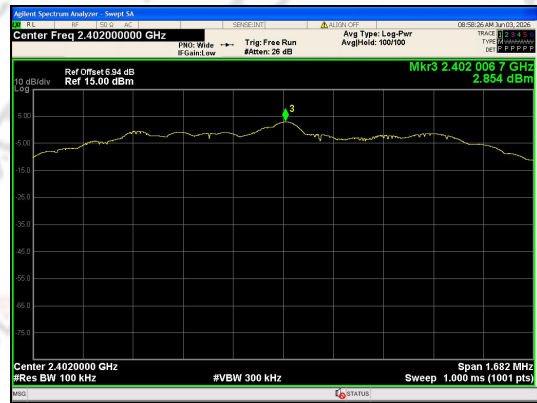
In-Band Reference Level BLE 2M_Channel 0
