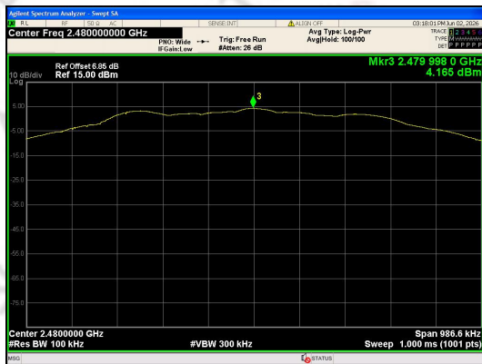
In-Band Reference Level BLE 1M_Channel 39
