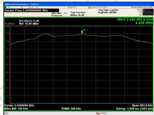
In-Band Reference Level LE Coded (S=8)_Channel 19
