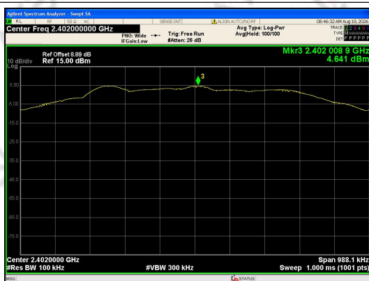
In-Band Reference Level LE Coded (S=2)_Channel 0
