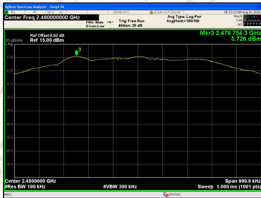
In-Band Reference Level LE Coded (S=2)_Channel 39
