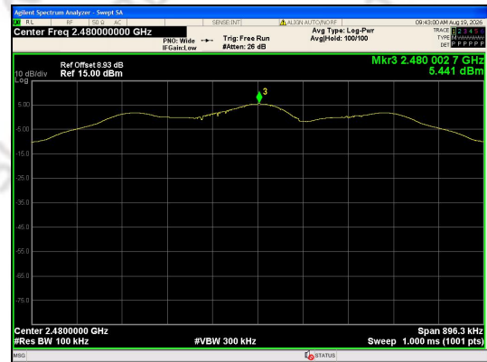
In-Band Reference Level LE Coded (S=8)_Channel 39
