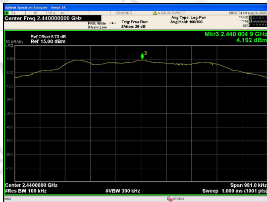
In-Band Reference Level LE Coded (S=2)_Channel 19
