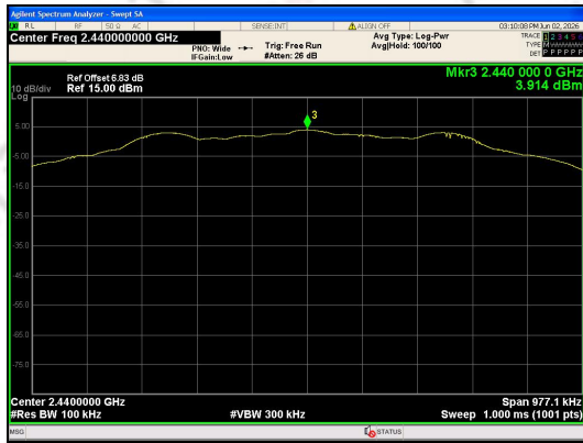
In-Band Reference Level BLE 1M_Channel 19
