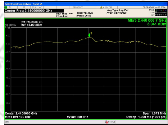
In-Band Reference Level BLE 2M_Channel 19
