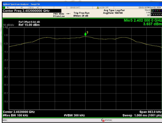
In-Band Reference Level BLE 1M_Channel 0
