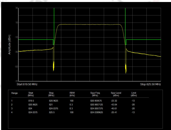
Band26(814-824) QAM16 BW=3MHz Channel=26775 RB Size=15
