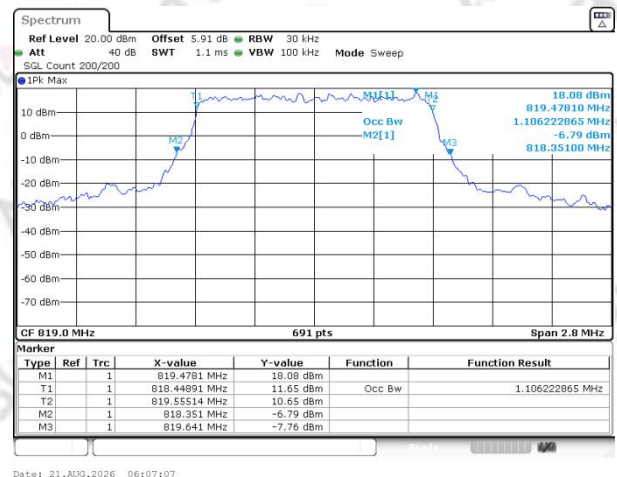
Band26(814-824) QPSK BW=1.4MHz Channel=26740 RB Size=6 Position=#0
