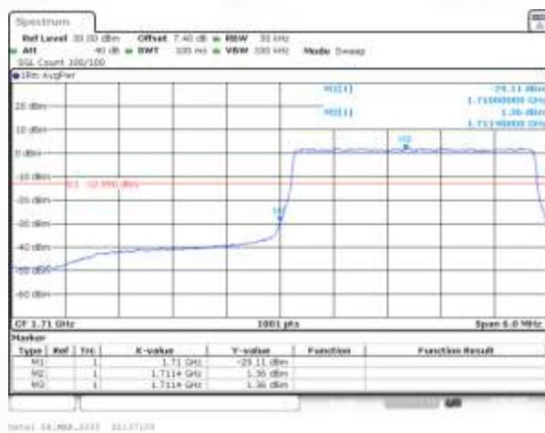
Band4 QPSK BW=3MHz Channel=19965 RB Size=15 Position=#0
