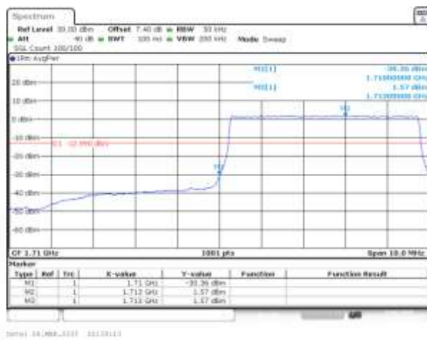
Band4 QPSK BW=5MHz Channel=19975 RB Size=25 Position=#0
