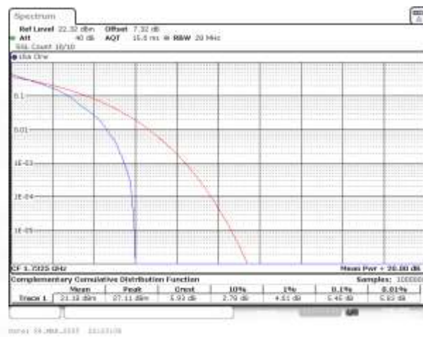
Band4 QPSK BW=5MHz Channel=20175 RB Size=1 Position=#0
