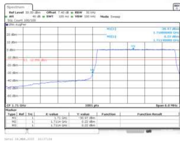
Band4 QAM16 BW=3MHz Channel=19965 RB Size=15 Position=#0
