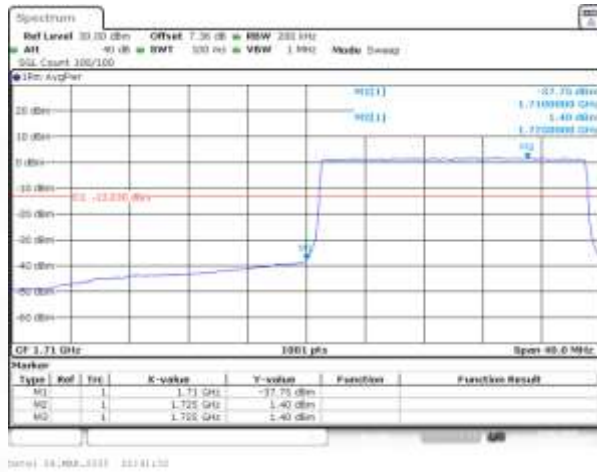
Band4 QPSK BW=20MHz Channel=20050 RB Size=100 Position=#0
