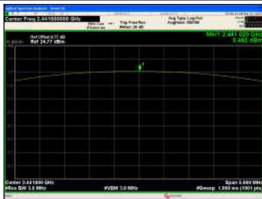
Peak Output Power GFSK_Channel 39
