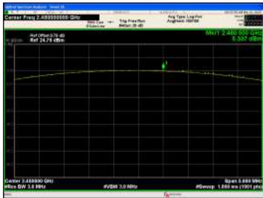
Peak Output Power \pi/4 DQPSK_Channel 78
