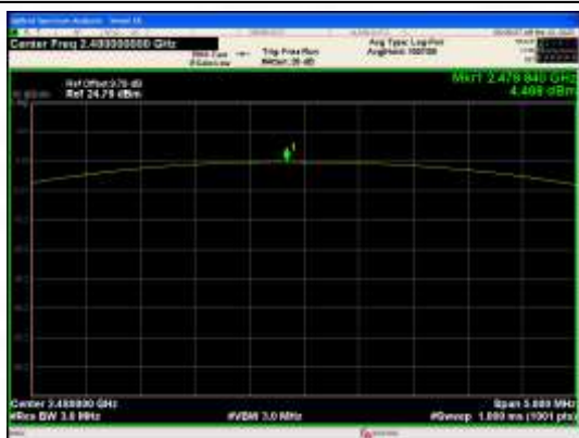
Peak Output Power GFSK_Channel 78
