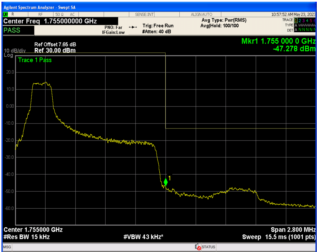
Band4 QPSK BW=1.4MHz Channel=20393 RB Size=6 Position=#0
