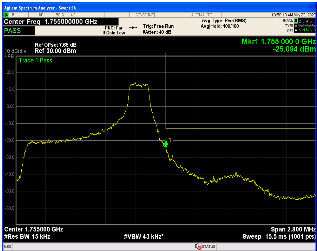
Band4 QPSK BW=3MHz Channel=19965 RB Size=1 Position=#0
