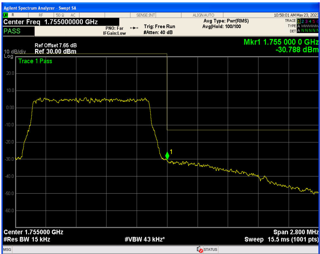
Band4 16QAM BW=1.4MHz Channel=20393 RB Size=1 Position=#0
