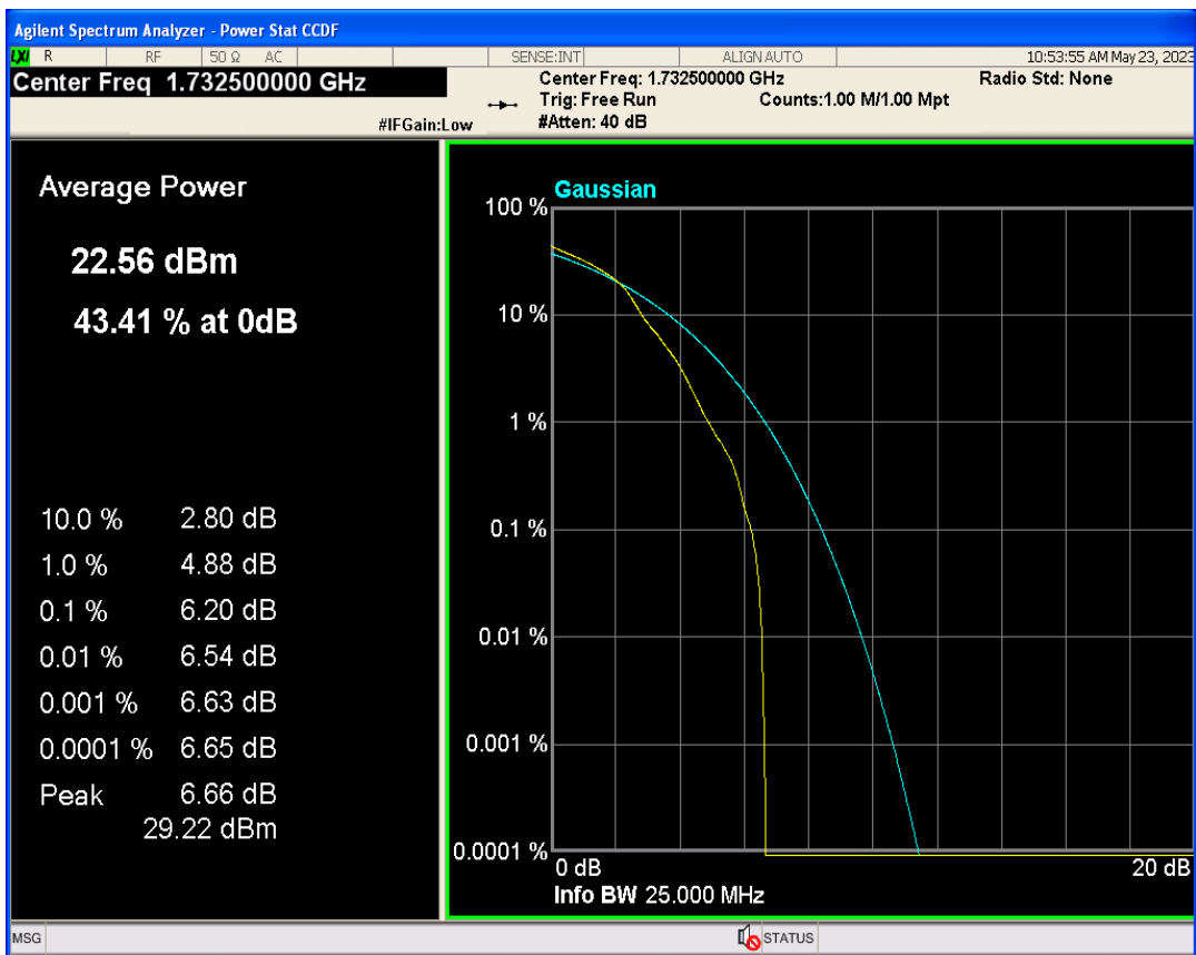
Band4 QPSK BW=10MHz Channel=20175 RB Size=1 Position=#0
