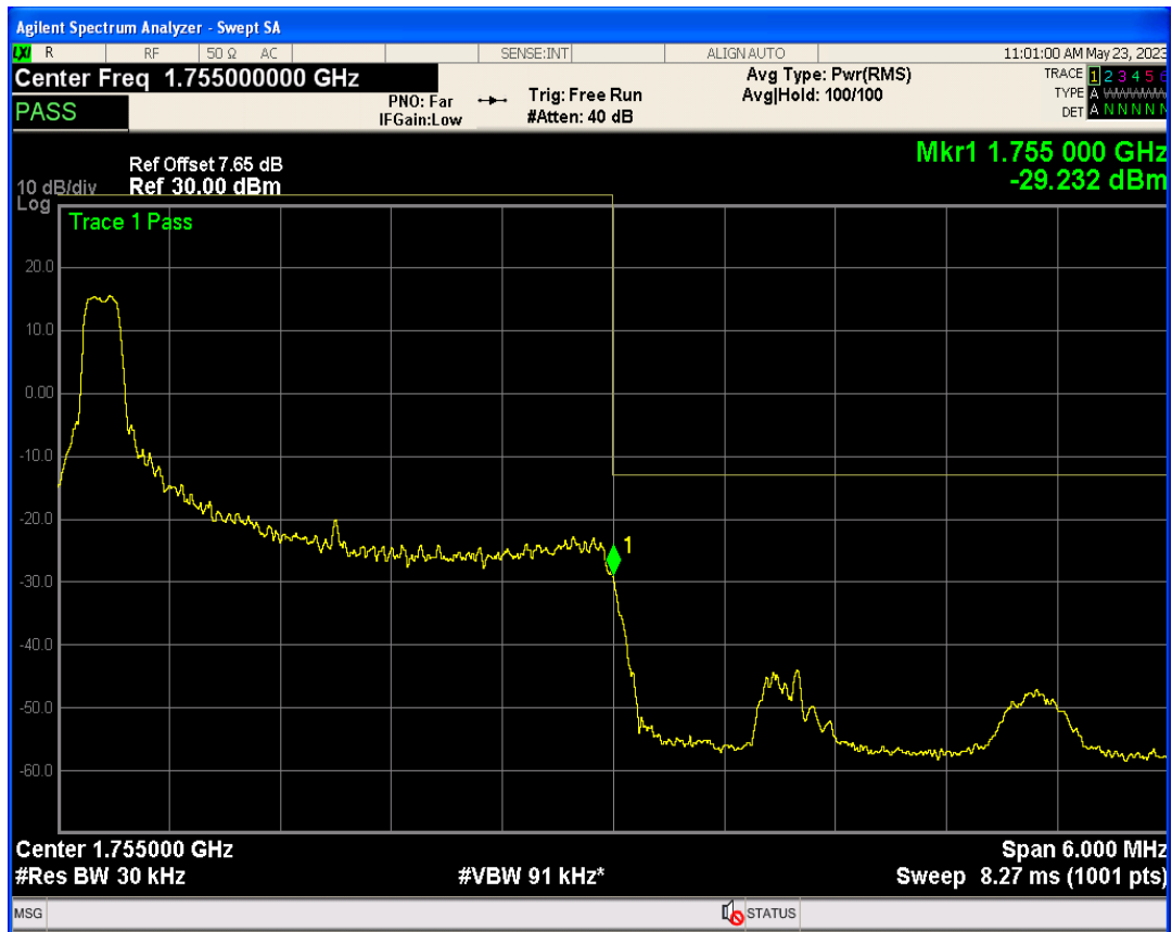
Band4 16QAM BW=3MHz Channel=20385 RB Size=15 Position=#0
