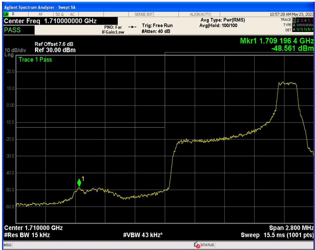
Band4 QPSK BW=1.4MHz Channel=19957 RB Size=6 Position=#0
