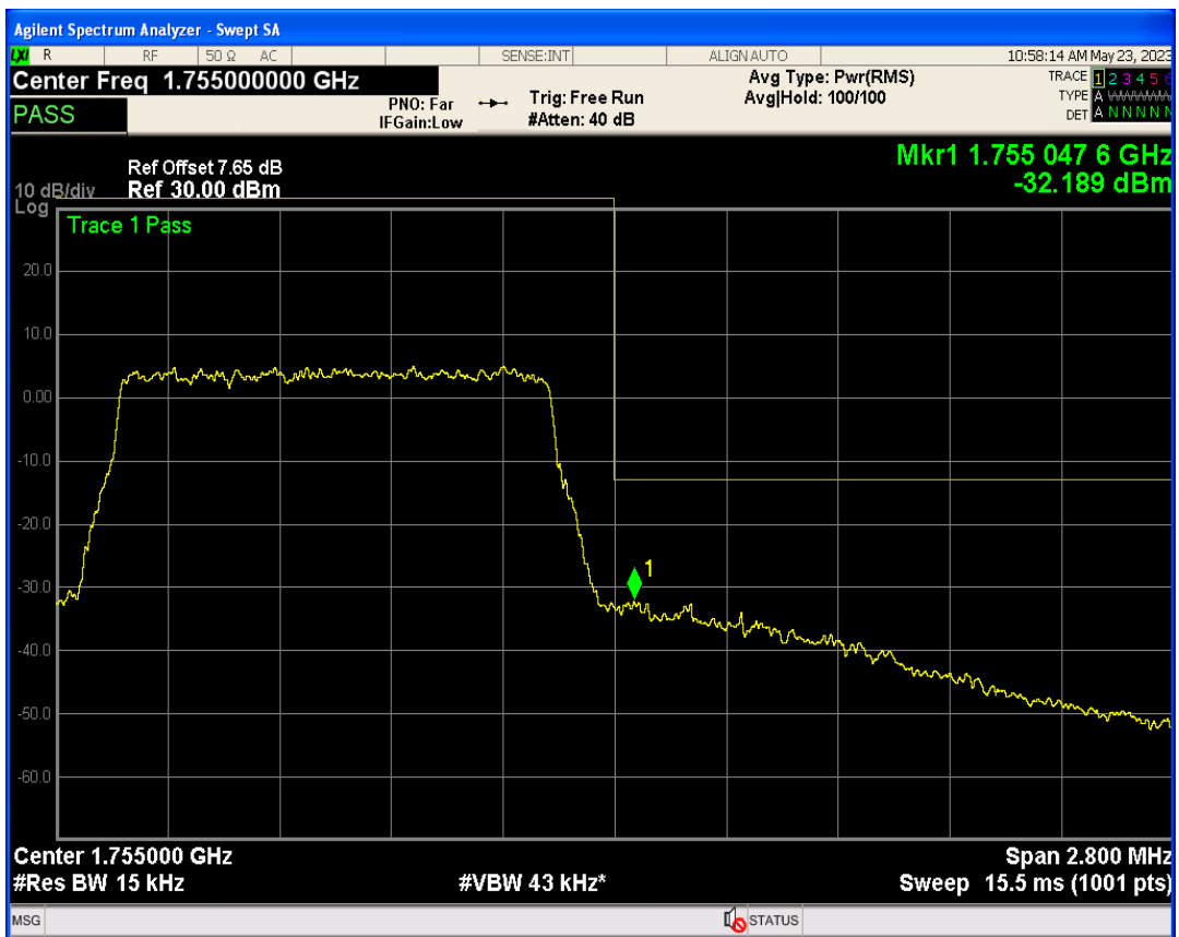
Band4 QPSK BW=3MHz Channel=19965 RB Size=1 Position=#Max
