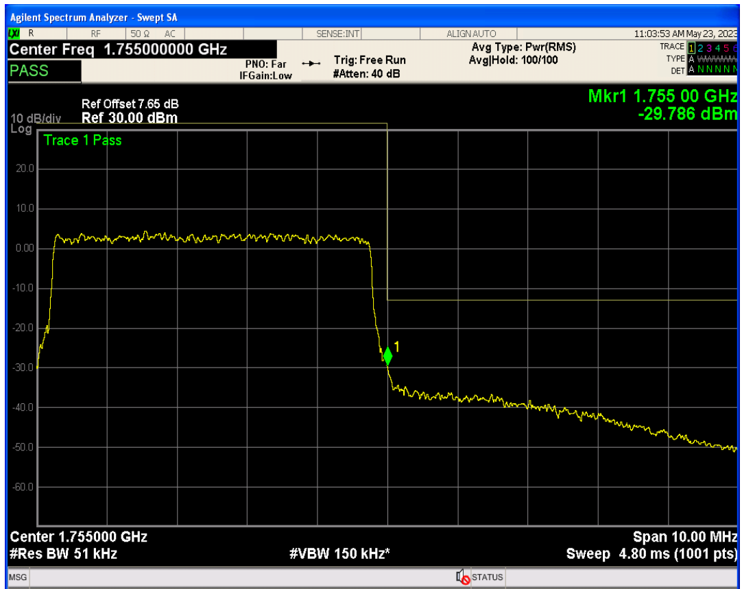
Band4 QPSK BW=10MHz Channel=20000 RB Size=1 Position=#Max
