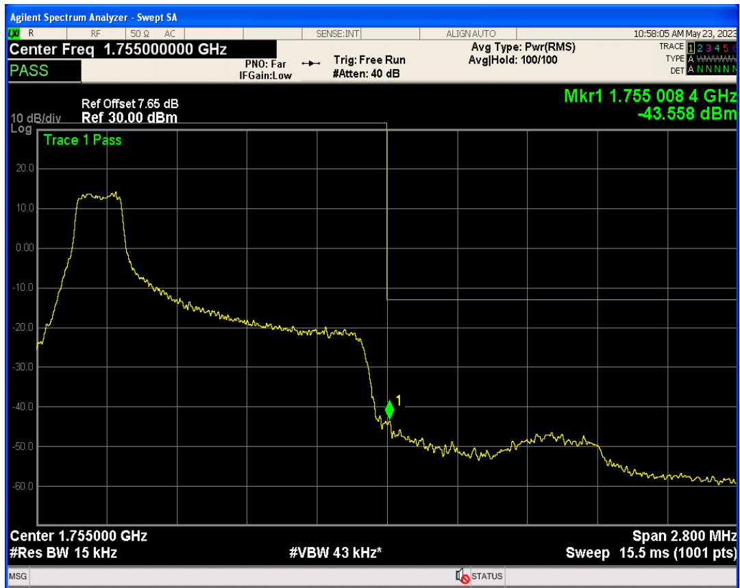
Band4 16QAM BW=1.4MHz Channel=20393 RB Size=1 Position=#Max
