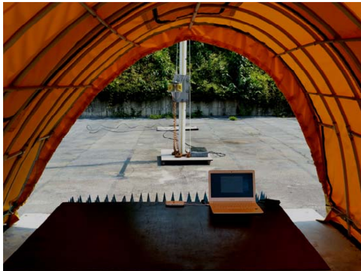
Photograph 2 : Setup for radiated Emissions (above 1 GHz)
