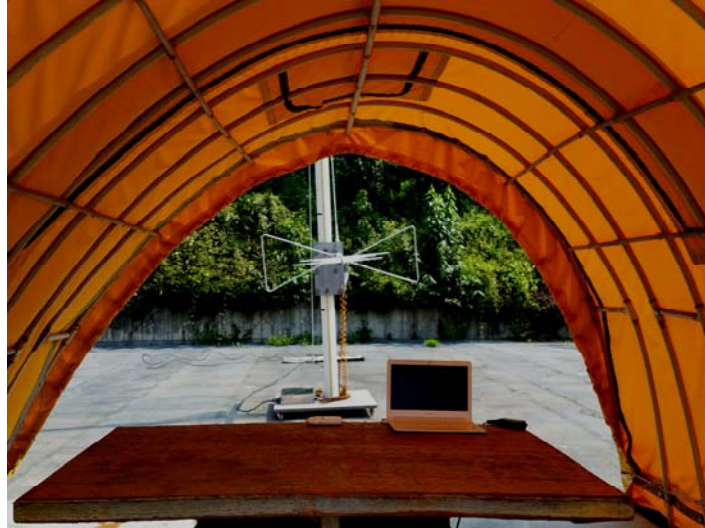
Photograph 2 : Setup for radiated Emissions (above 1 GHz)
