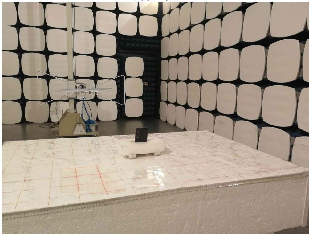
Radiated Spurious Emission Below 1GHz
