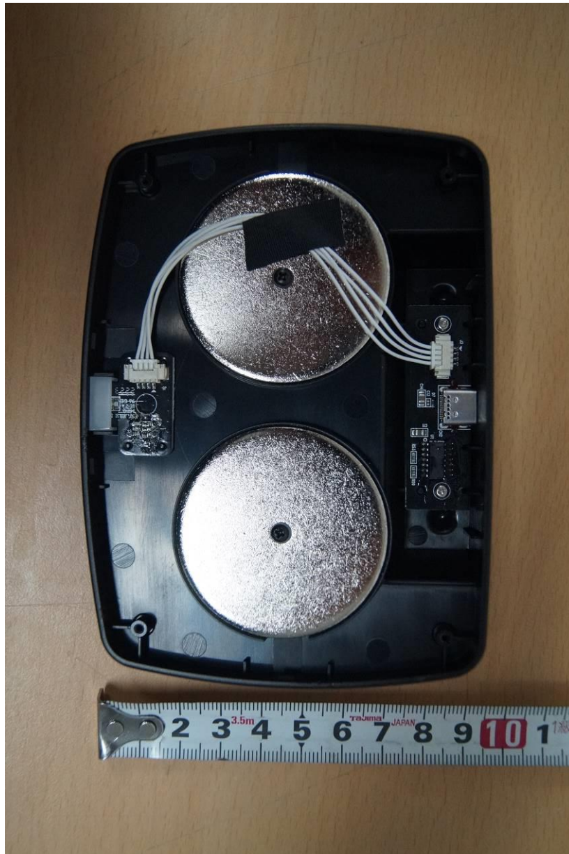
< Charging cradle inside view >
