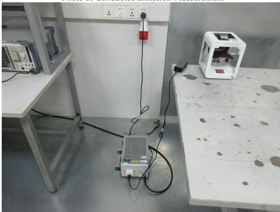
Photo of Conducted Emission Measurement
