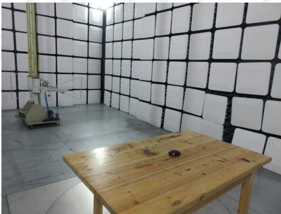
Photo of Radiation Emission Test
