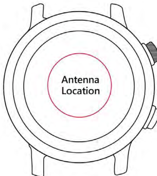
Fig.7 Antenna location (front view)
