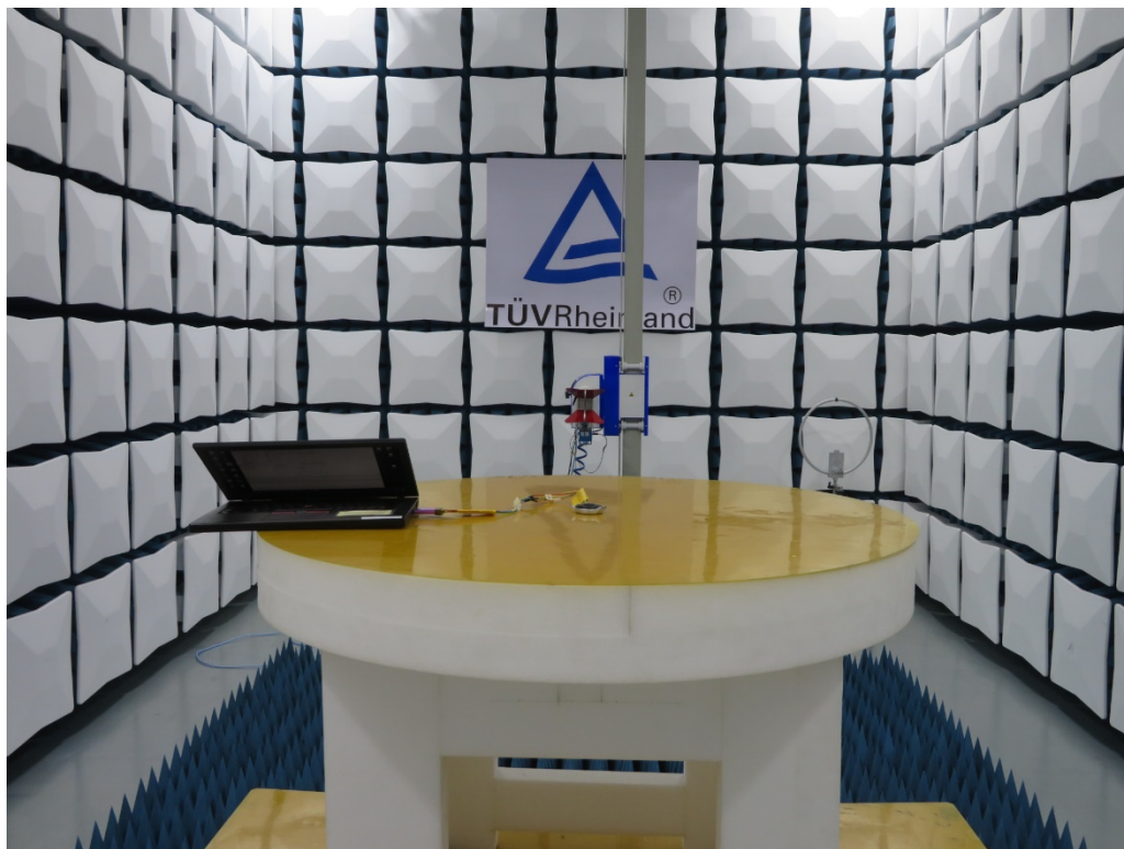
Photograph 2: Set-up for Radiated Spurious Emission, Above 1GHz
