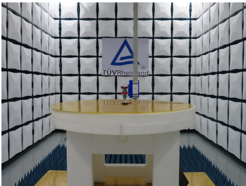
Photograph 2: Set-up for Radiated Spurious Emission, Above 1GHz
