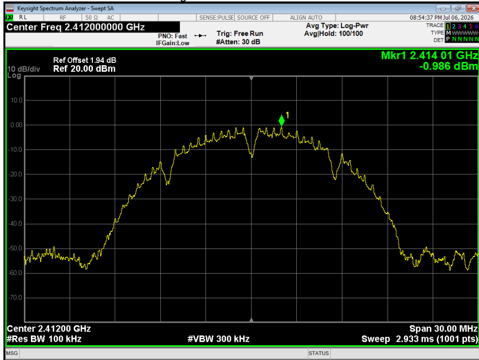
Band Edge NVNT b 2412MHz Ant1 Emission
