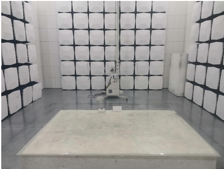
RADIATED EMISSION MEASUREMENT (below 1G)
