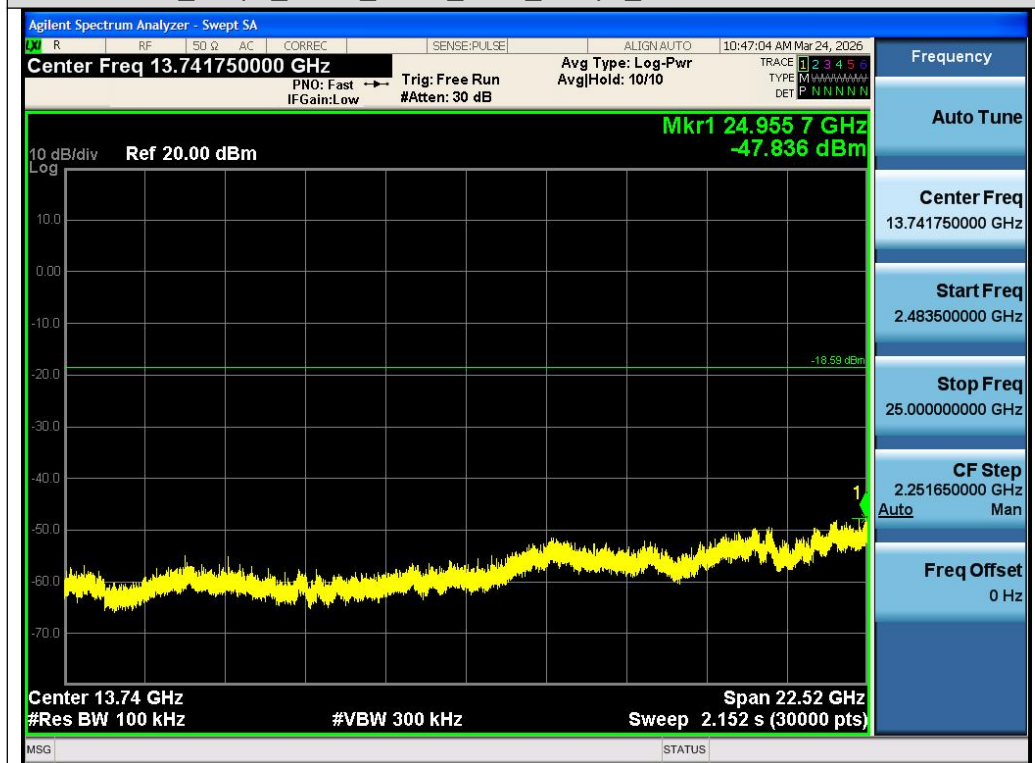
Test_Graph_LE1M_ANT1_2440_1Mbps_Higher Band Emissions
