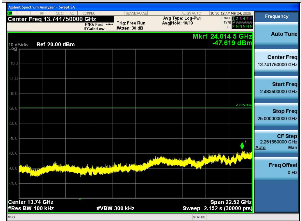
Test_Graph_LE2M_ANT1_2404_2Mbps_Higher Band Emissions
