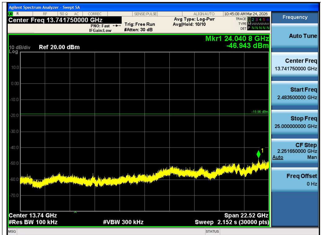
Test_Graph_LE2M_ANT1_2440_2Mbps_Higher Band Emissions
