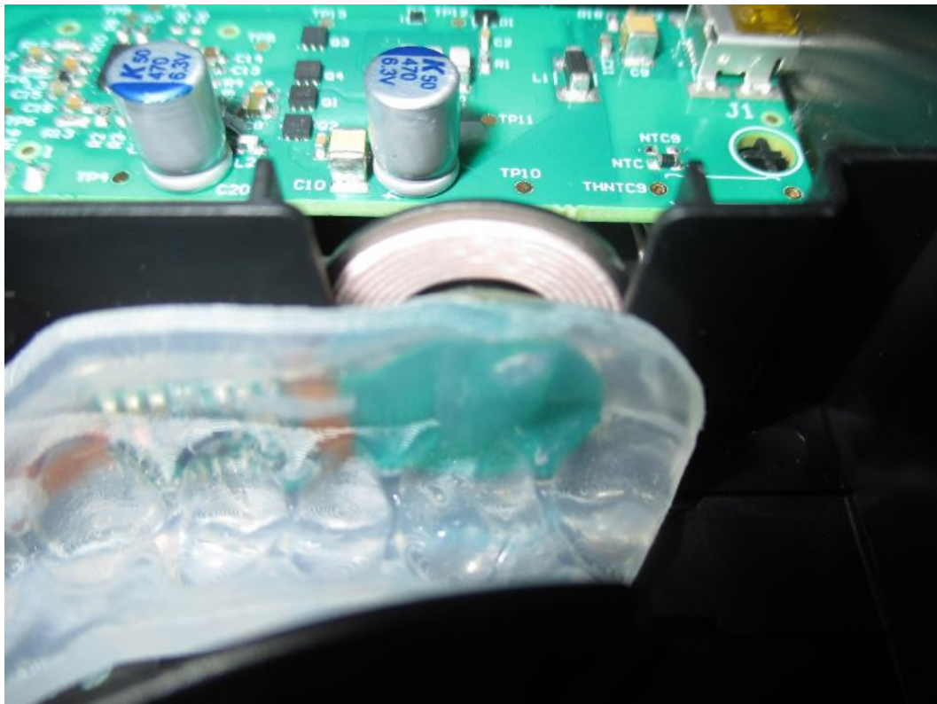
EUT with mouthguard in position 2 (best aligned position)
