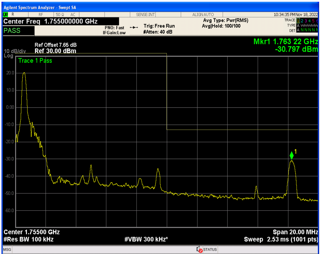
Band4 QAM16 BW=10MHz Channel=20350 RB Size=1 Position=#Max
