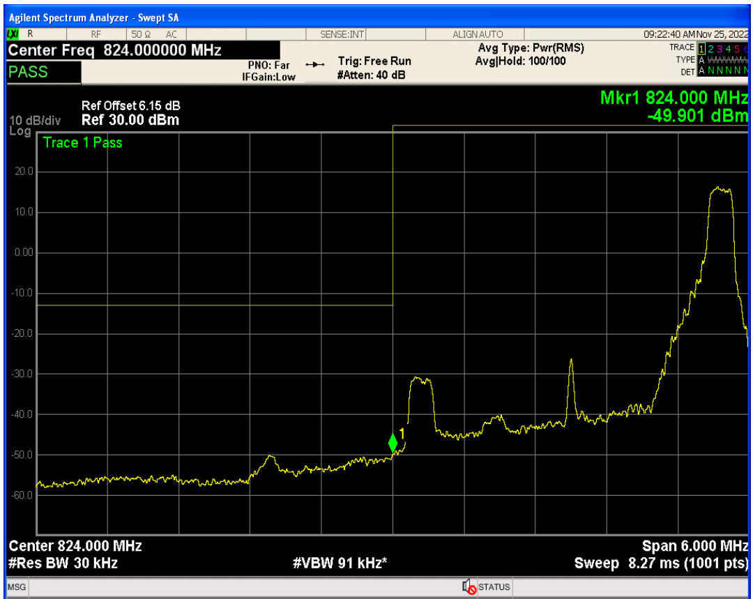
Band26b QAM16 BW=3MHz Channel=26805 RB Size=15 Position=#0
