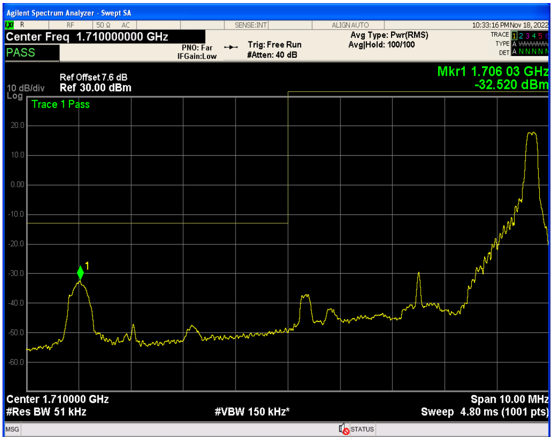
Band4 QPSK BW=5MHz Channel=19975 RB Size=25 Position=#0
