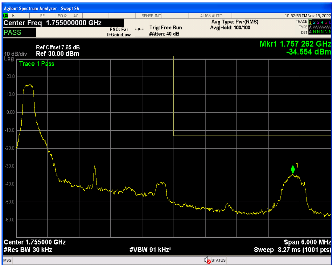
Band4 QAM16 BW=3MHz Channel=20385 RB Size=1 Position=#Max
