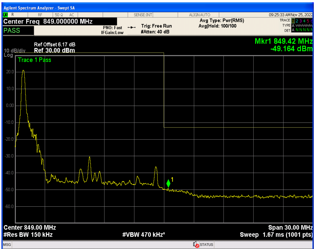
Band26b QAM16 BW=15MHz Channel=26965 RB Size=75 Position=#0
