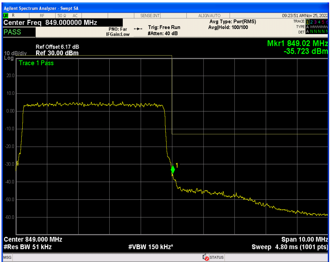
Band26b QAM16 BW=5MHz Channel=27015 RB Size=25 Position=#0
