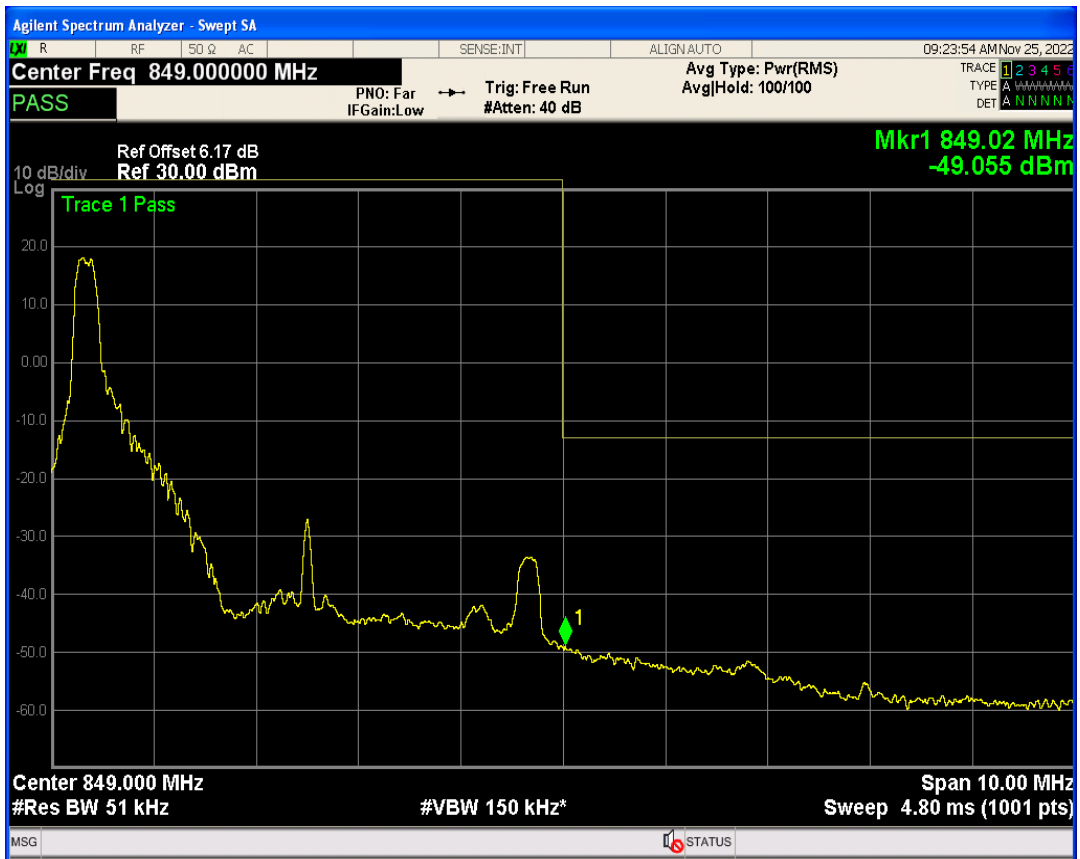
Band26b QPSK BW=5MHz Channel=27015 RB Size=25 Position=#0
