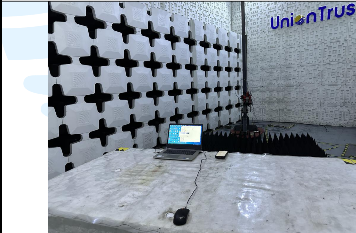
Radiated emission Test Setup (Above 1 GHz) _Test Mode 8
