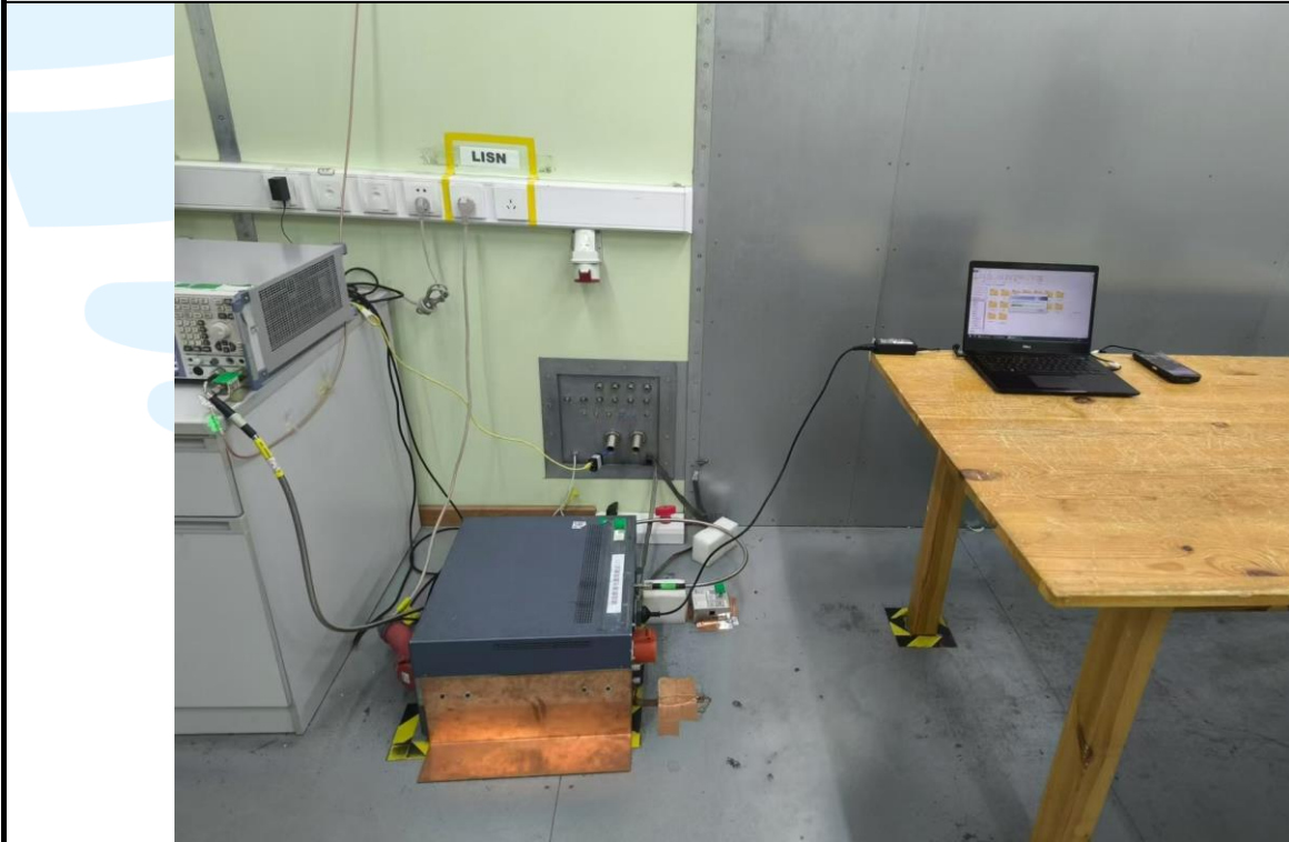
Conducted Emission Test Setup _Test Mode 7
