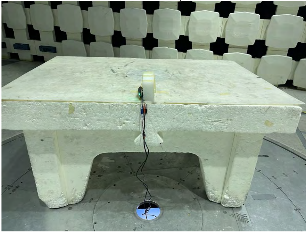
Radiated Emissions Test Setup, 30-1000 MHz
