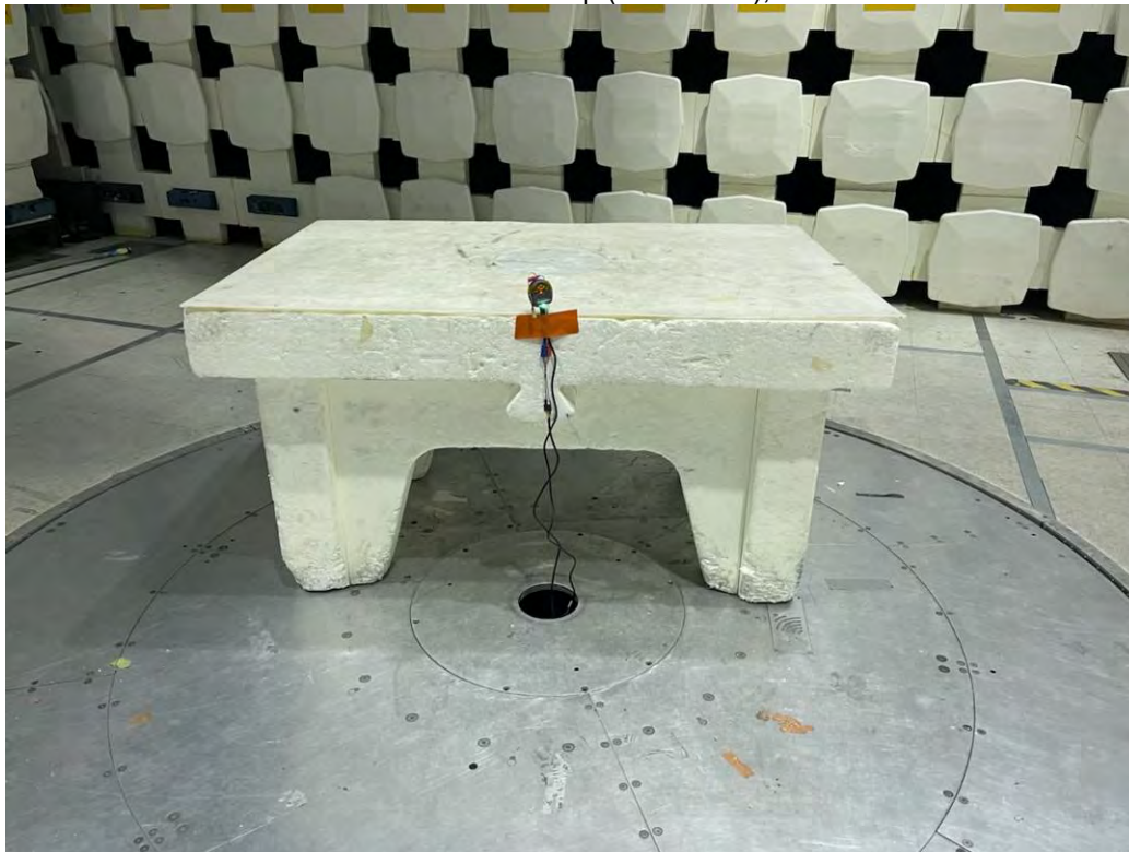
Radiated Emissions Test Setup (Short Side), 30-1000 MHz
