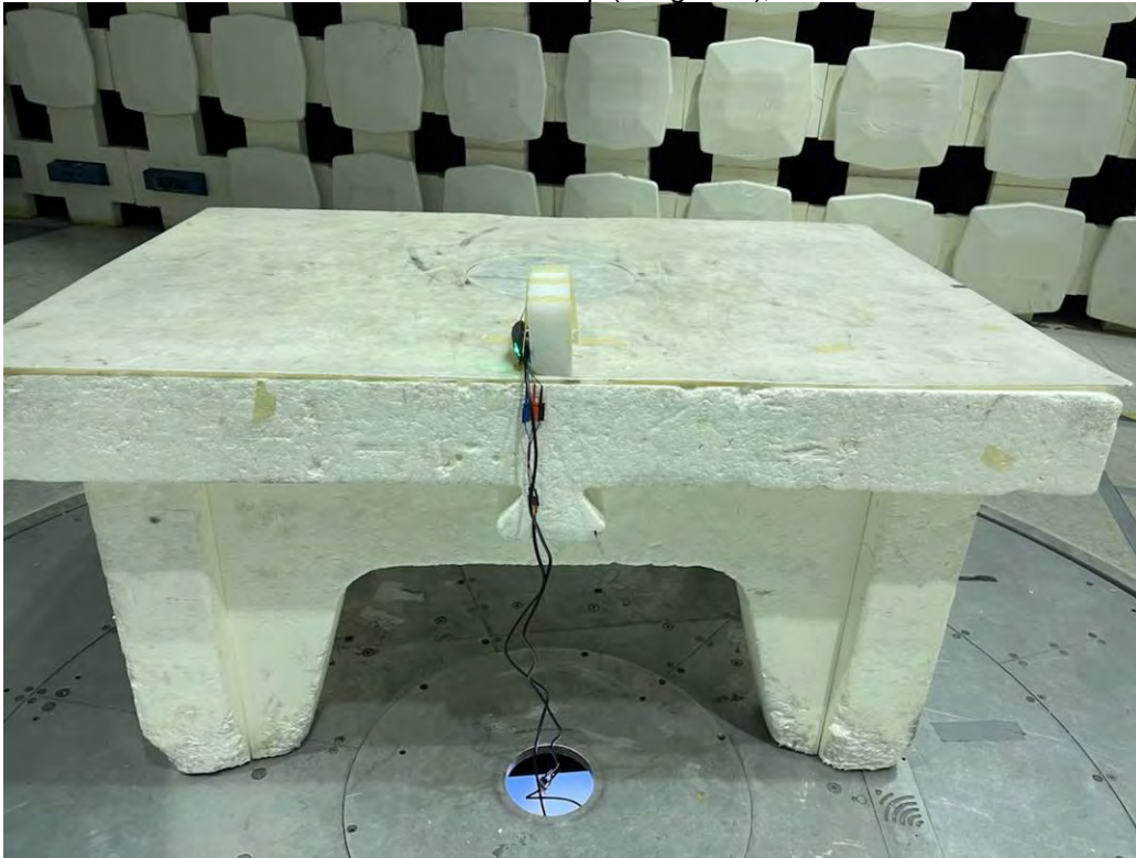
Radiated Emissions Test Setup (Long Side), 30-1000 MHz
