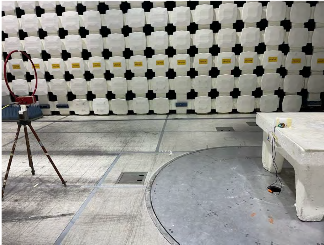
Radiated Emissions Test Setup, 9 kHz-30 MHz
