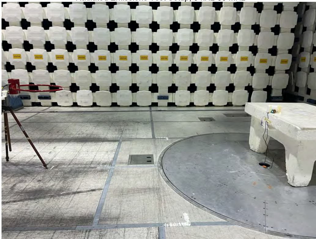
Radiated Emissions Test Setup, 9 kHz-30 MHz
