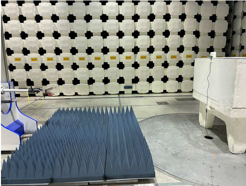
Radiated Emissions Test Setup, 1-13 GHz (Short Side)
