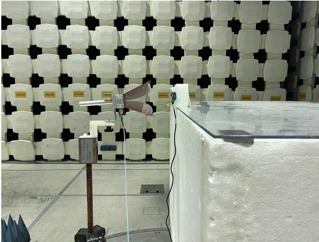
Radiated Emissions Manual Scan Test Setup, 18-25 GHz
