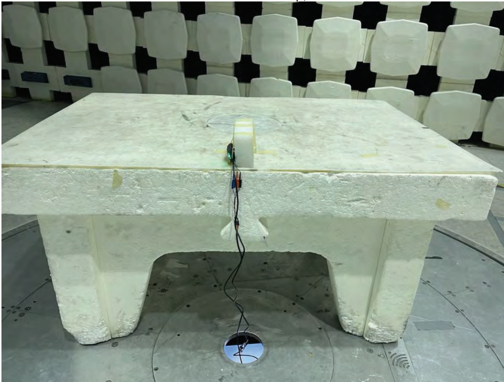
Radiated Emissions Test Setup, 30-1000 MHz
