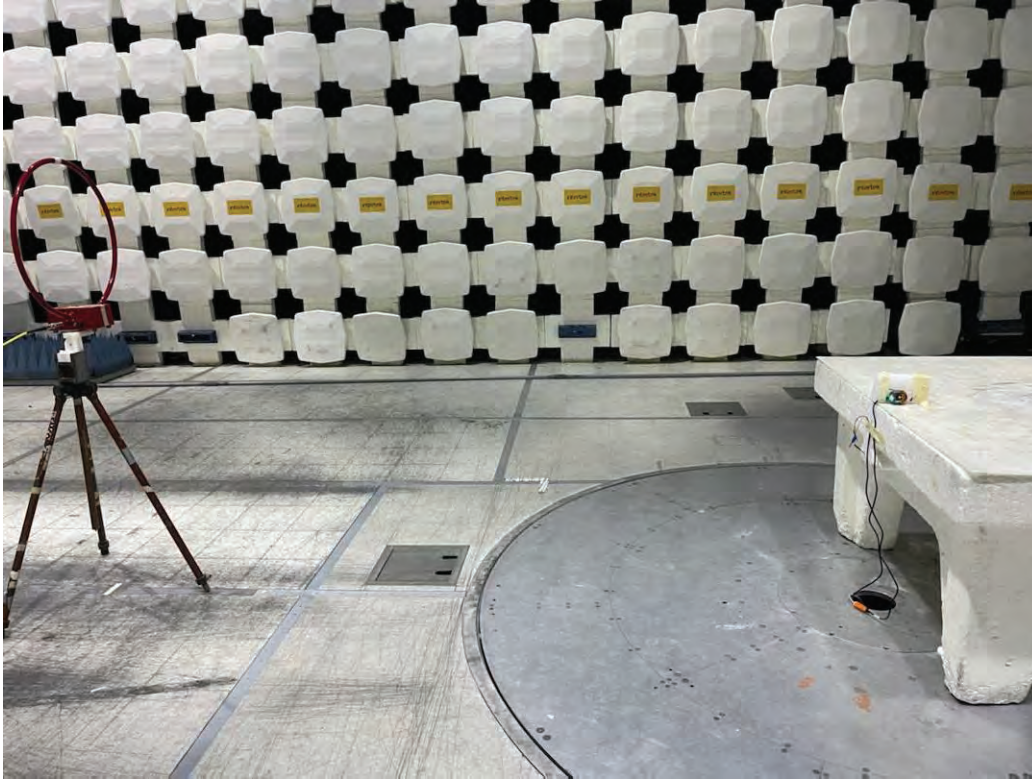
Radiated Emissions Test Setup, 9 kHz-30 MHz
