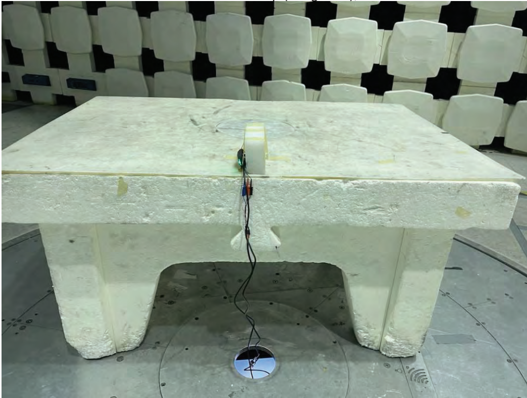
Radiated Emissions Test Setup (Long Side), 30-1000 MHz
