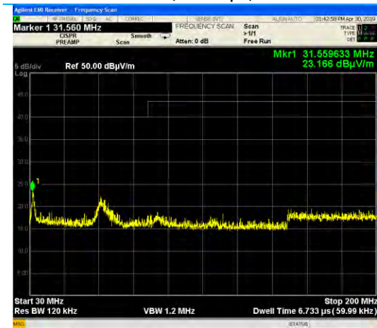
30-1000 MHz, Vertical EUT, Vertical Antenna 802.11b, 1 Mbps, Channel 11
