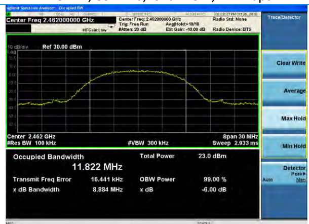
DTS BW, 802.11b, Channel 11, 11 Mbps
