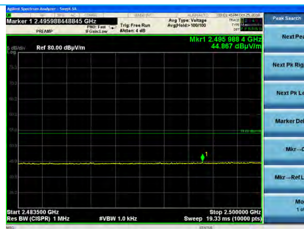
2483.5-2500 MHz, Side EUT, Horizontal Antenna 802.11n HT20, MCS0, Channel 1, Average
