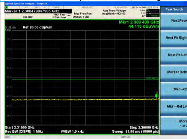
2310-2390 MHz, Side EUT, Horizontal Antenna 802.11g, 6 Mbps, Channel 1, Average
