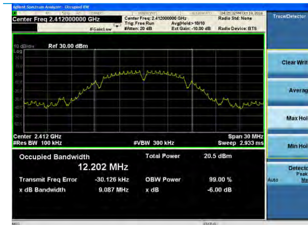
DTS BW, 802.11b, Channel 1, 1 Mbps
