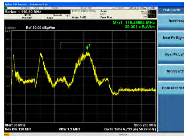
30-1000 MHz, Vertical EUT, Horizontal Antenna 802.11b, 1 Mbps, Channel 1
