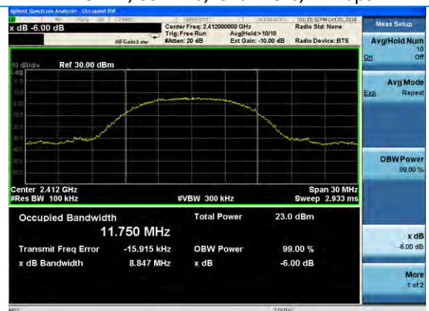
DTS BW, 802.11b, Channel 1, 11 Mbps
