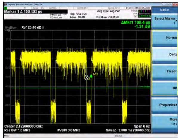
Duty Cycle, 802.11n HT40, MCS0, Off Time
