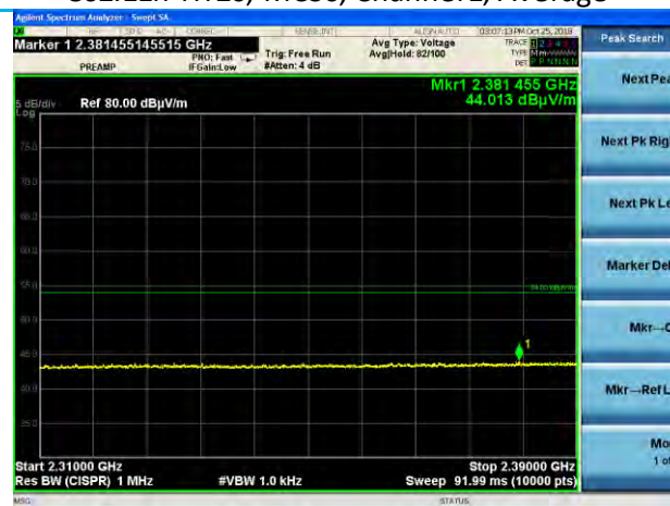
2310-2390 MHz, Side EUT, Horizontal Antenna 802.11n HT20, MCS7, Channel 1, Average
