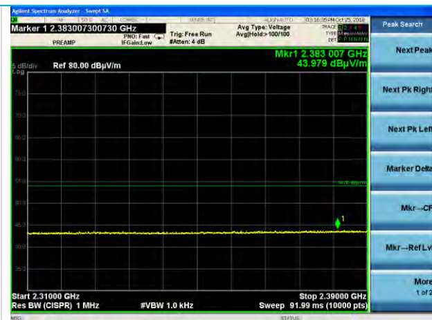
2310-2390 MHz, Side EUT, Horizontal Antenna 802.11n HT40, MCS0, Channel3, Average
