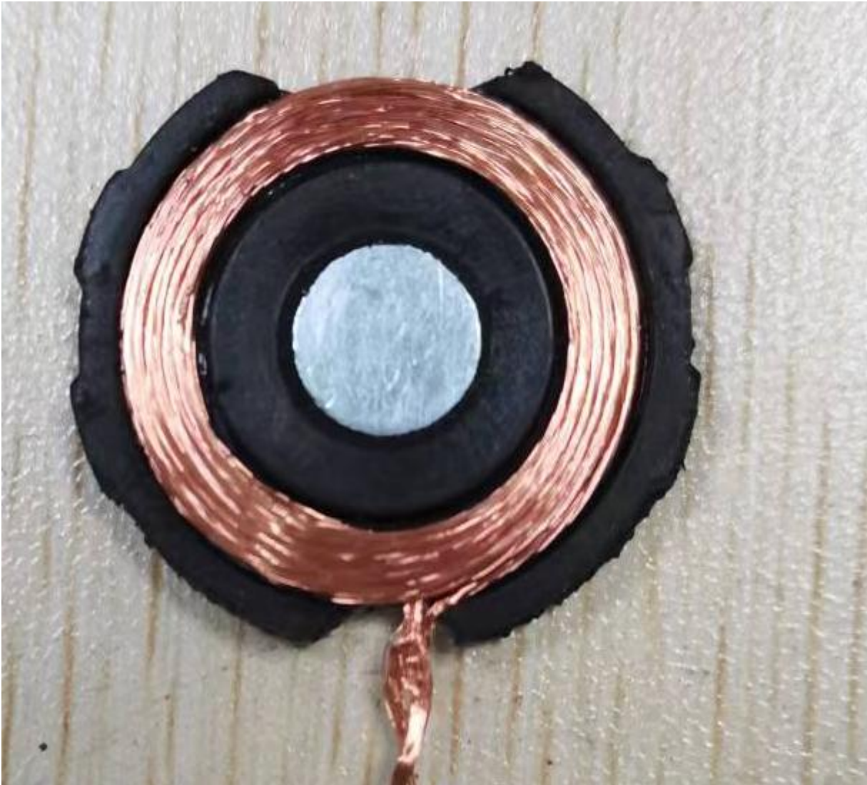
Antenna type: Inductive loop coil Antenna, 0dBi
