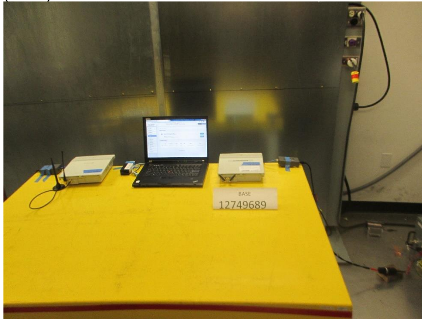
(BASE) LINE CONDUCTED FRONT PHOTO
