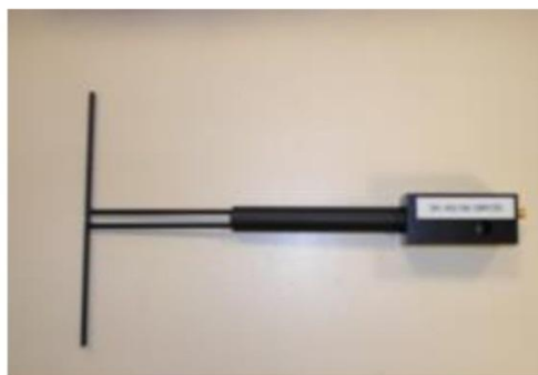
Figure 1 – Satimo COMOSAR Validation Dipole
