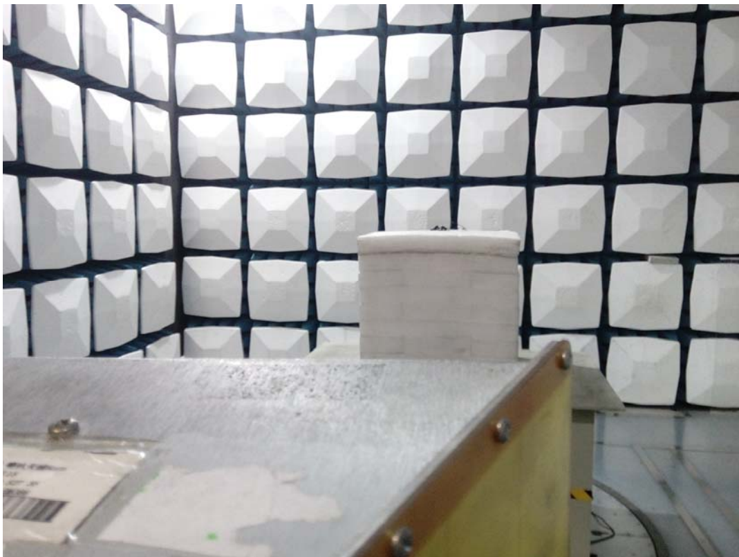
Radiated Emission Above 1GHz View
