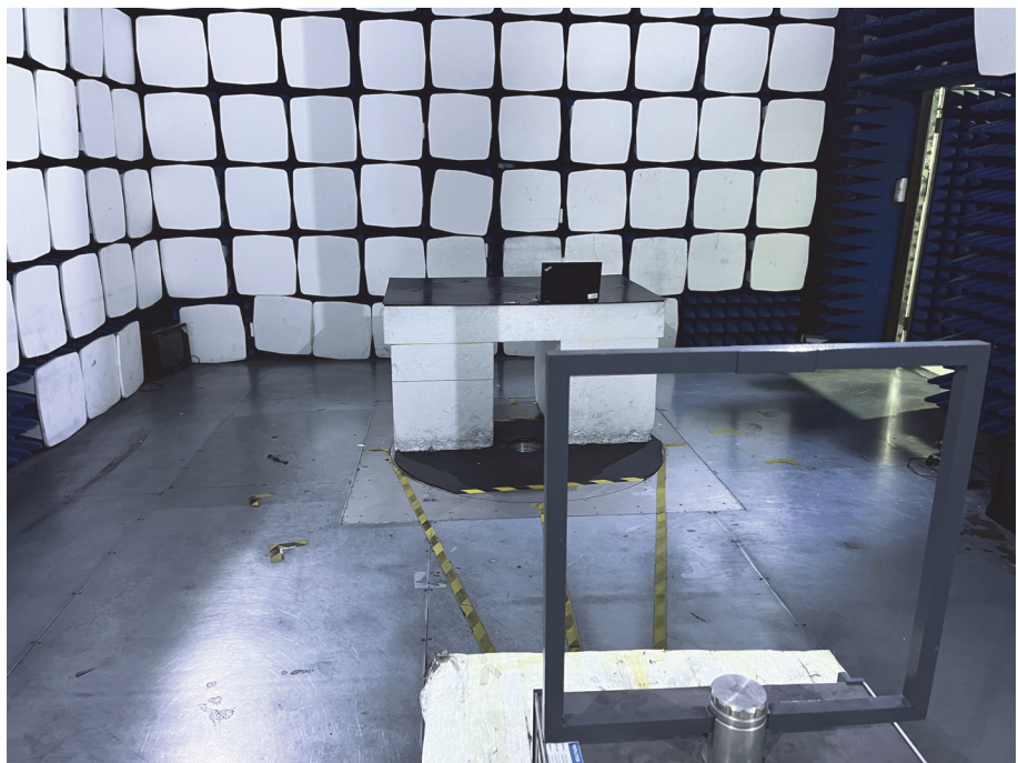
Radiation Emission Test Setup (Below 30MHz)
