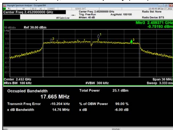
802.11n(HT20), Carrier frequency (MHz): 2452
