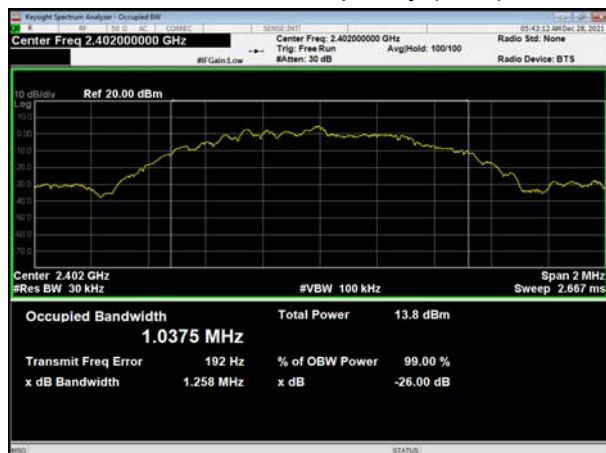
Bluetooth LE Carrier frequency (MHz): 2402
