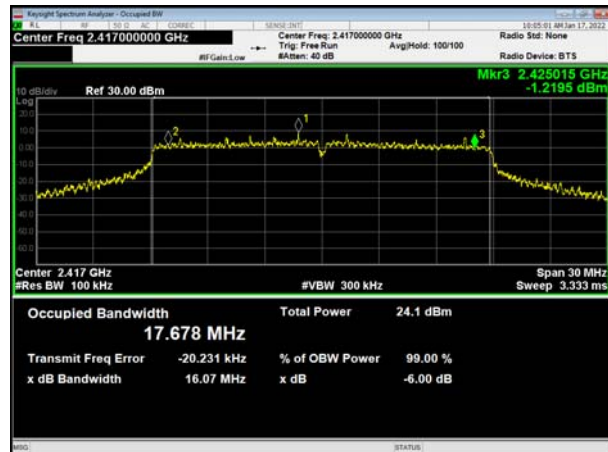
802.11n(HT20), Carrier frequency (MHz): 2417
