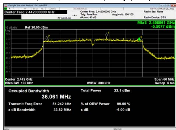
802.11n(HT40), Carrier frequency (MHz): 2442
