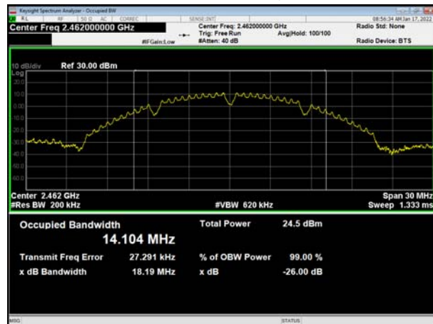
802.11b, Carrier frequency (MHz): 2462
