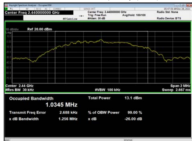
Bluetooth LE Carrier frequency (MHz): 2440
