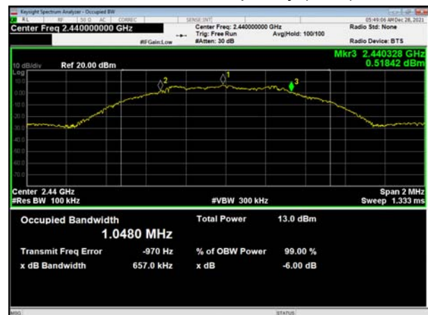
Bluetooth LE Carrier frequency (MHz): 2440
