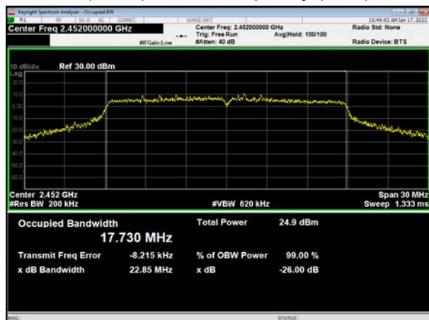
802.11n(HT20), Carrier frequency (MHz): 2452
