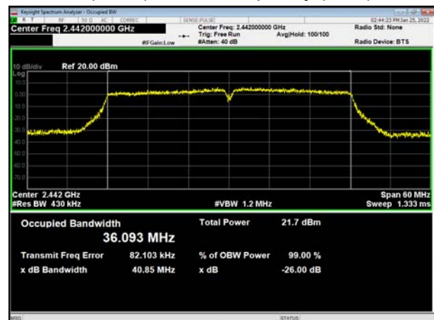
802.11n(HT40), Carrier frequency (MHz): 2442
