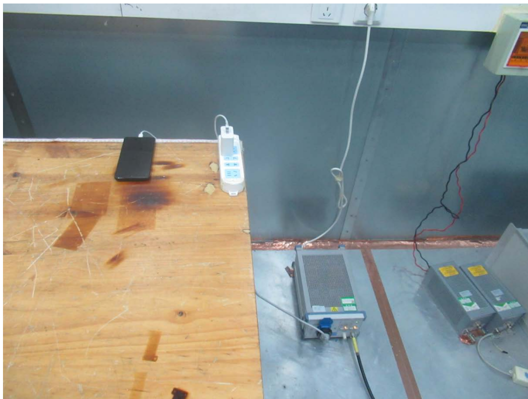
Picture 2 Conducted Emission Test Setup
