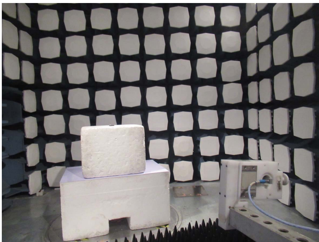
Picture 1 Radiated Emission Test Setup
