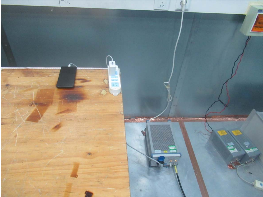
Picture 2 Conducted Emission Test Setup
