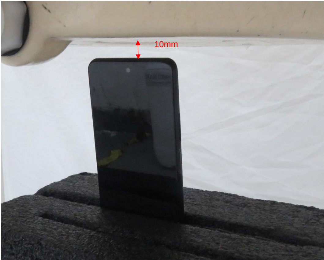
Picture 11: Top Side, the distance from handset to the bottom of the Phantom is 10mm
