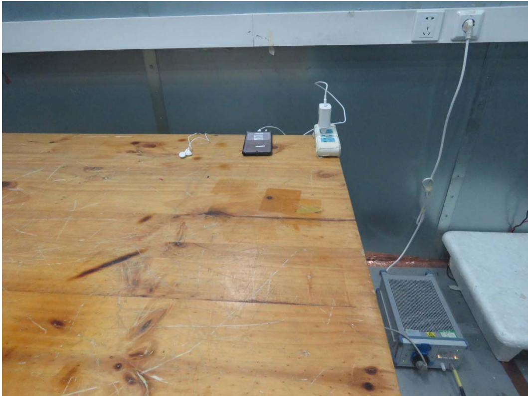
Picture 2 Conducted Emission Test Setup
