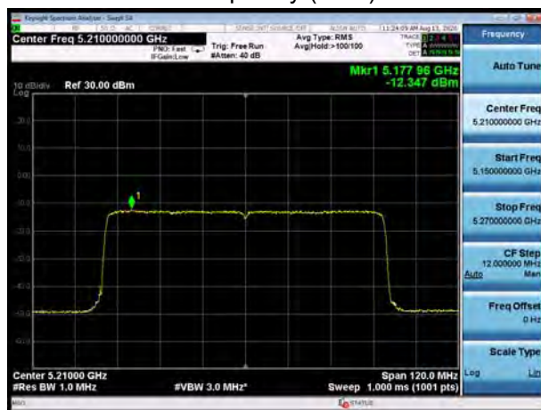
U-NII-1, 802.11ax HE80 Carrier frequency (MHz): 5210
