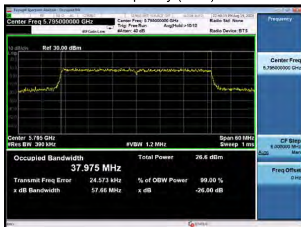
U-NII-3, 802.11ax HE80 Carrier frequency (MHz):5775
