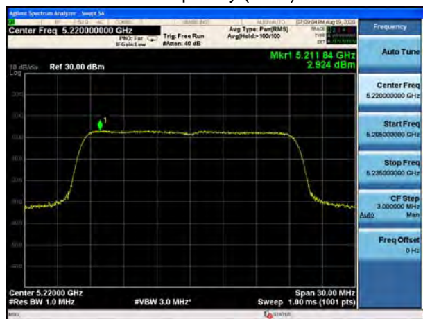
U-NII-1, 802.11ax HE20 Carrier frequency (MHz): 5220
