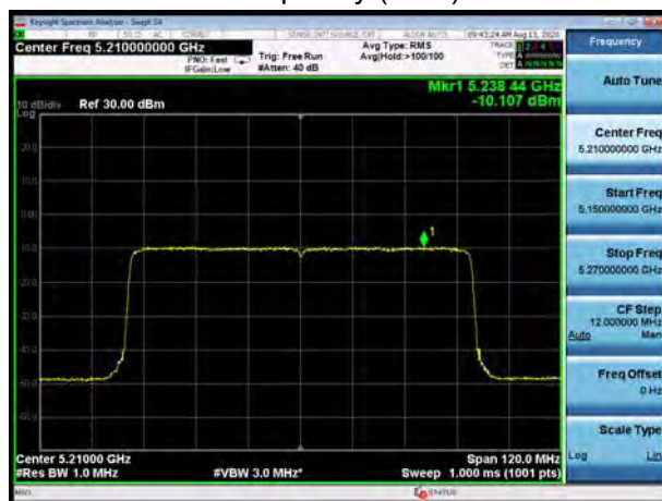
U-NII-1, 802.11ax HE80 Carrier frequency (MHz): 5210
