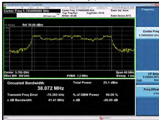
U-NII-3, 802.11ax HE80 Carrier frequency (MHz):5775
