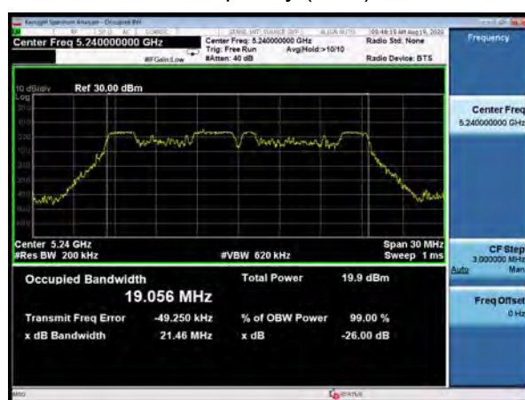
U-NII-1, 802.11ax HE20 Carrier frequency (MHz): 5240
