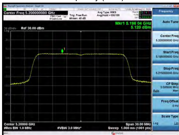
U-NII-1, 802.11ax HE20 Carrier frequency (MHz): 5220
