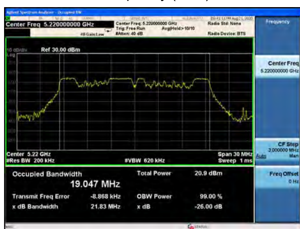
U-NII-1, 802.11ax HE20 Carrier frequency (MHz): 5220
