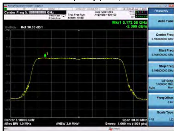
U-NII-1, 802.11ax HE20 Carrier frequency (MHz): 5200
