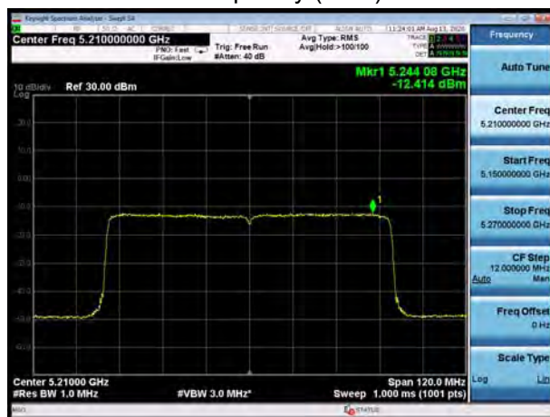
U-NII-1, 802.11ax HE80 Carrier frequency (MHz): 5210
