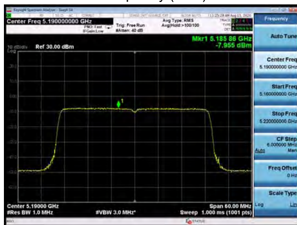
U-NII-1, 802.11ax HE40 Carrier frequency (MHz): 5230
