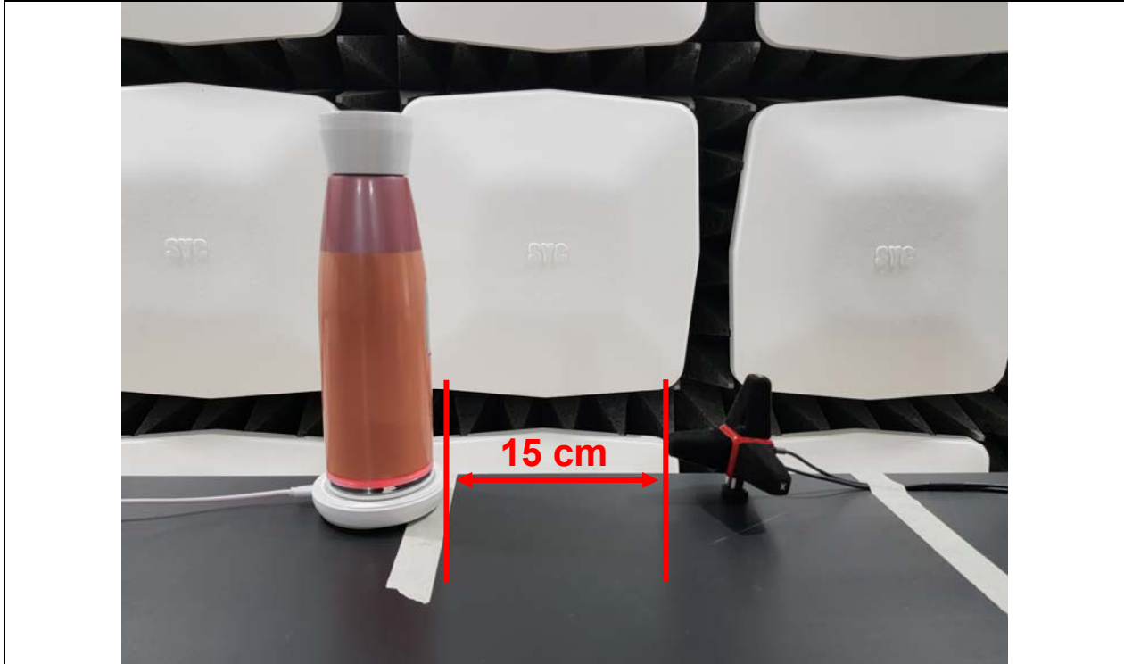
E-field Measurements _ Distance : 15 cm
