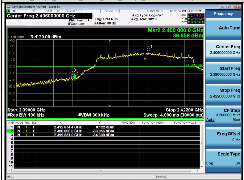
Test_Graph_802.11g_ANT1_2412_6Mbps_Lower Band Edge Emissions
