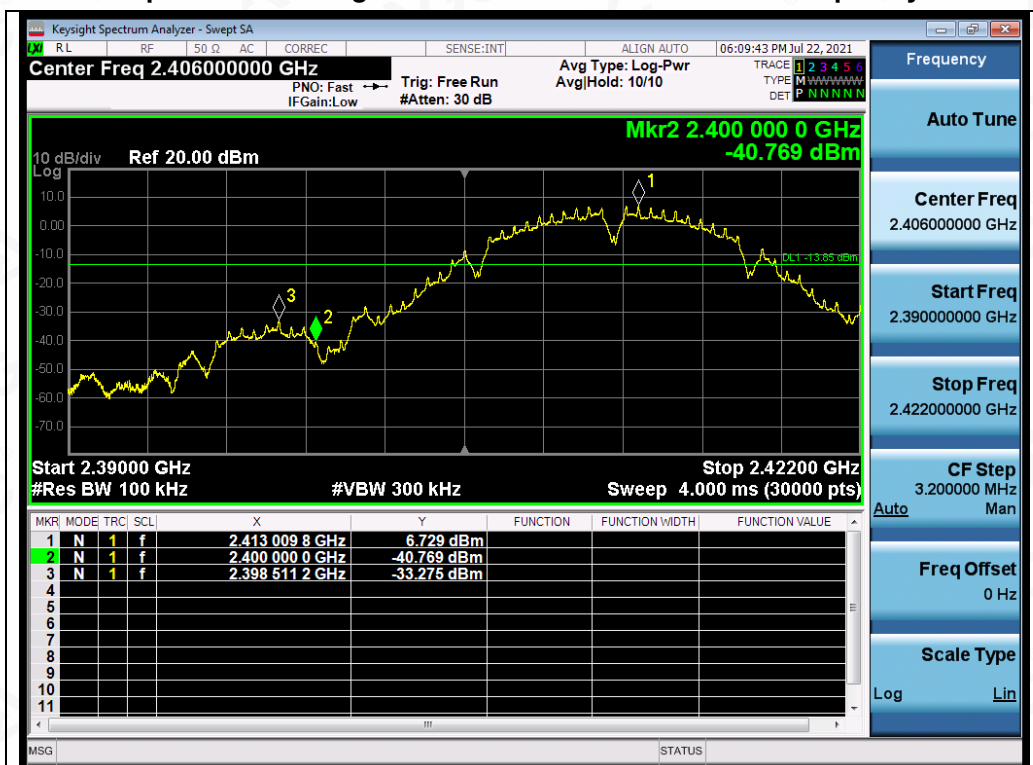
Test_Graph_802.11b_ANT1_2412_1Mbps_Lower Band Edge Emissions
