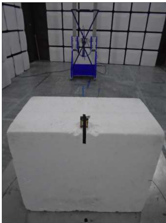
Figure 64 - Test Setup - 30 MHz to 1 GHz - Y Orientation
