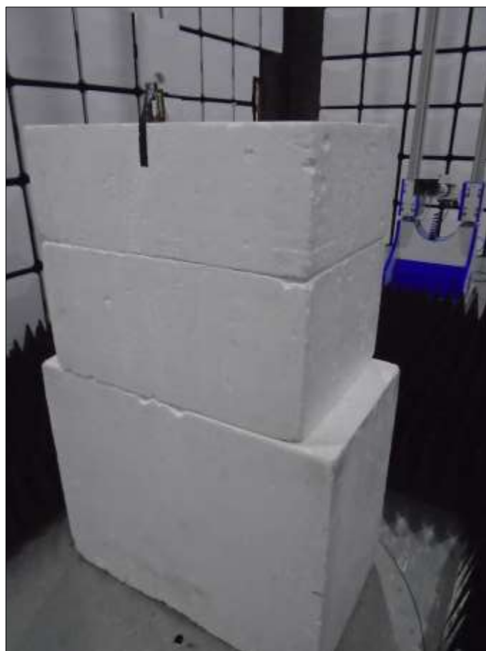
Figure 67 - Test Setup - 1 GHz to 10 GHz - Y Orientation
