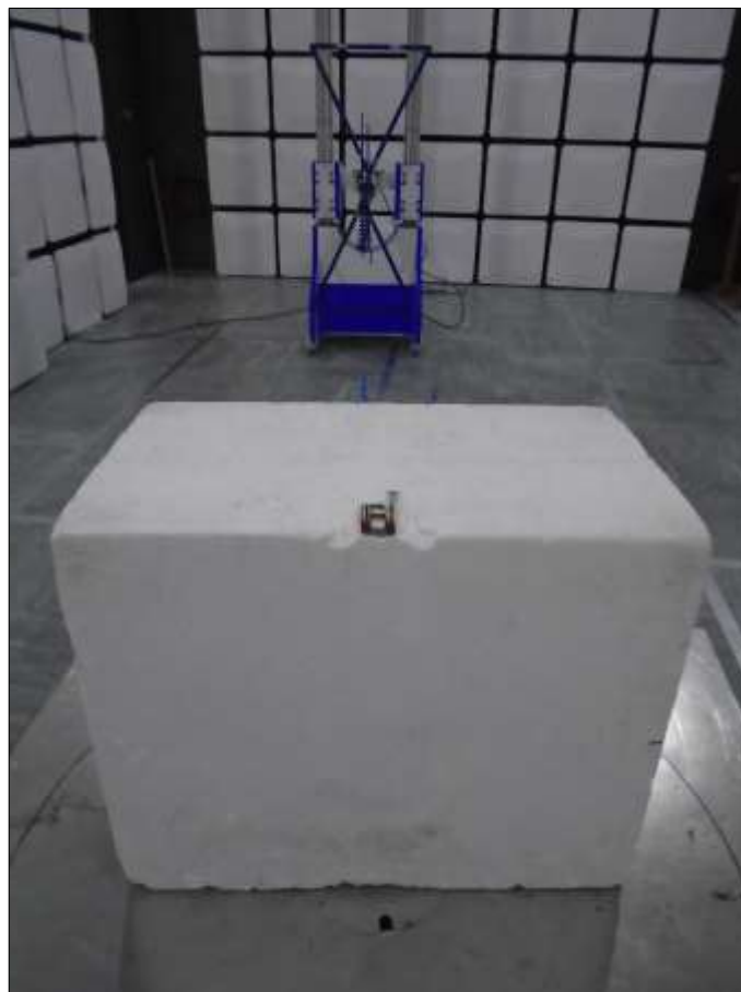
Figure 63 - Test Setup - 30 MHz to 1 GHz - X Orientation
