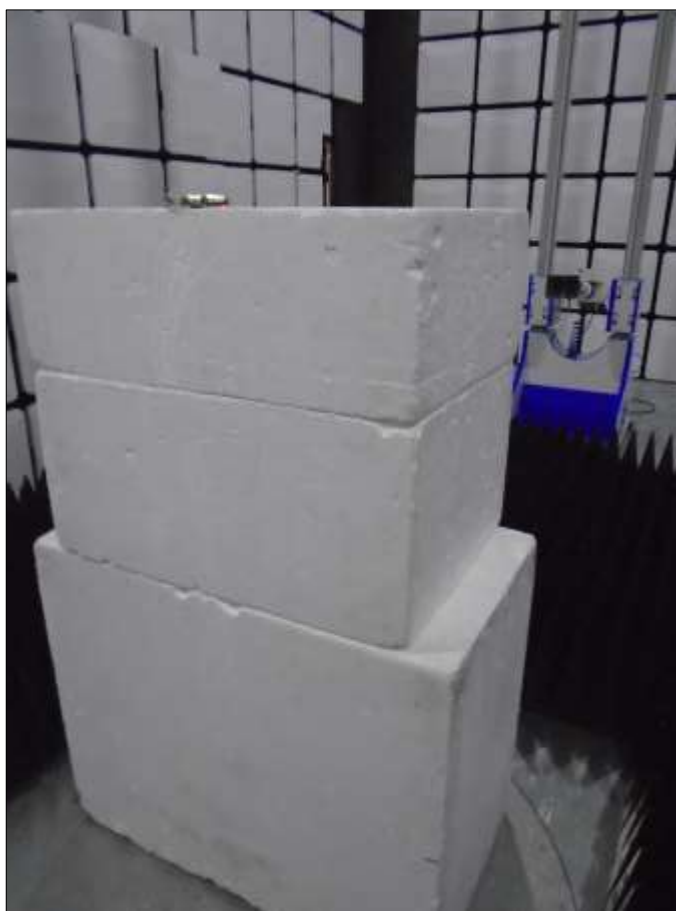
Figure 66 - Test Setup - 1 GHz to 10 GHz - X Orientation
