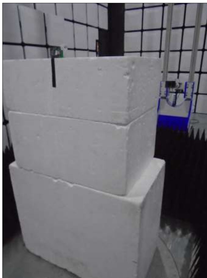
Figure 68 - Test Setup - 1 GHz to 10 GHz - Z Orientation
