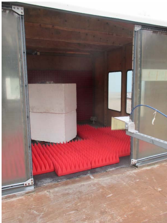
Vertical Antenna Polarization
