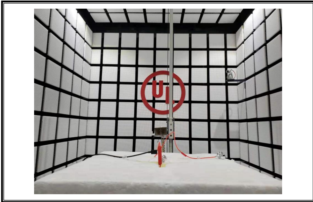
POWERLINE CONDUCTED EMISSIONS MEASUREMENT SETUP
