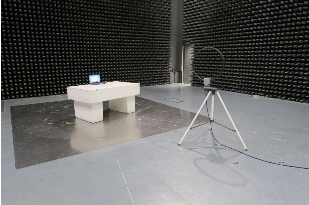
Photo 4.7.1 .....: Measurement of band edge SA3-USB
