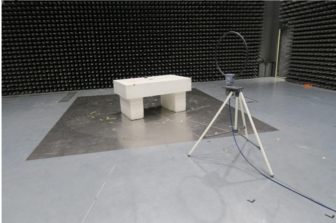
Photo 4.7.2 .....: Measurement of band edge SA3-D
