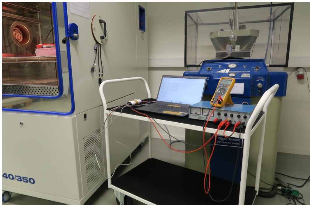
Photo 4.5.2 ..... Measurement of frequency stability
