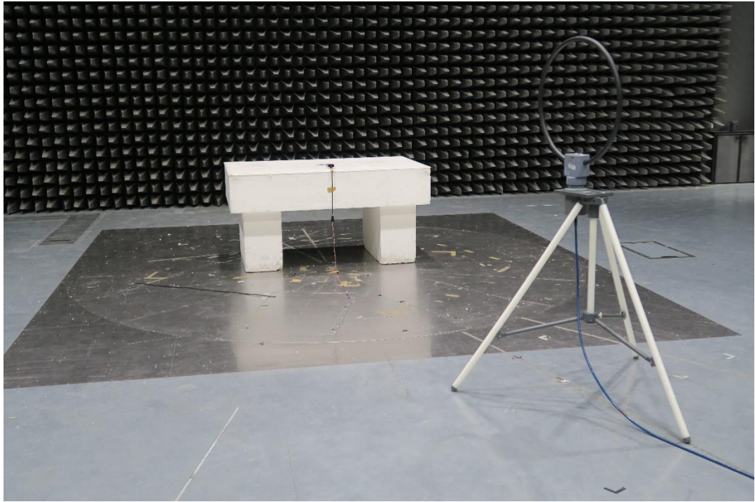
Photo 4.8.4.....: Measurement of field strength of fundamental SA3-F
