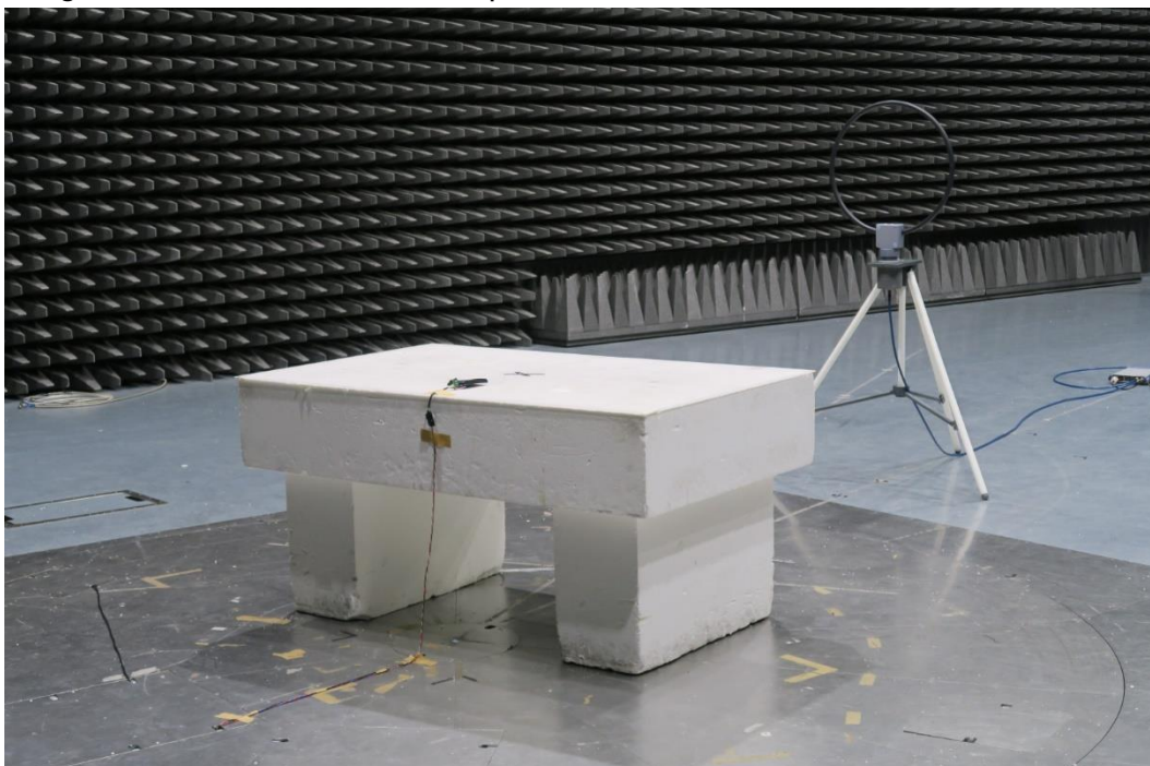
a. High angle front view of EUT on setup table, antenna axis X
