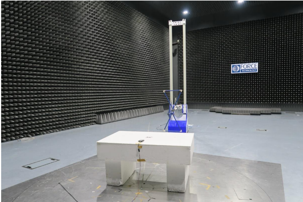
Photo 4.3.3.....: Measurement of Radiated emission 30 - 1000 MHz SA3-I
