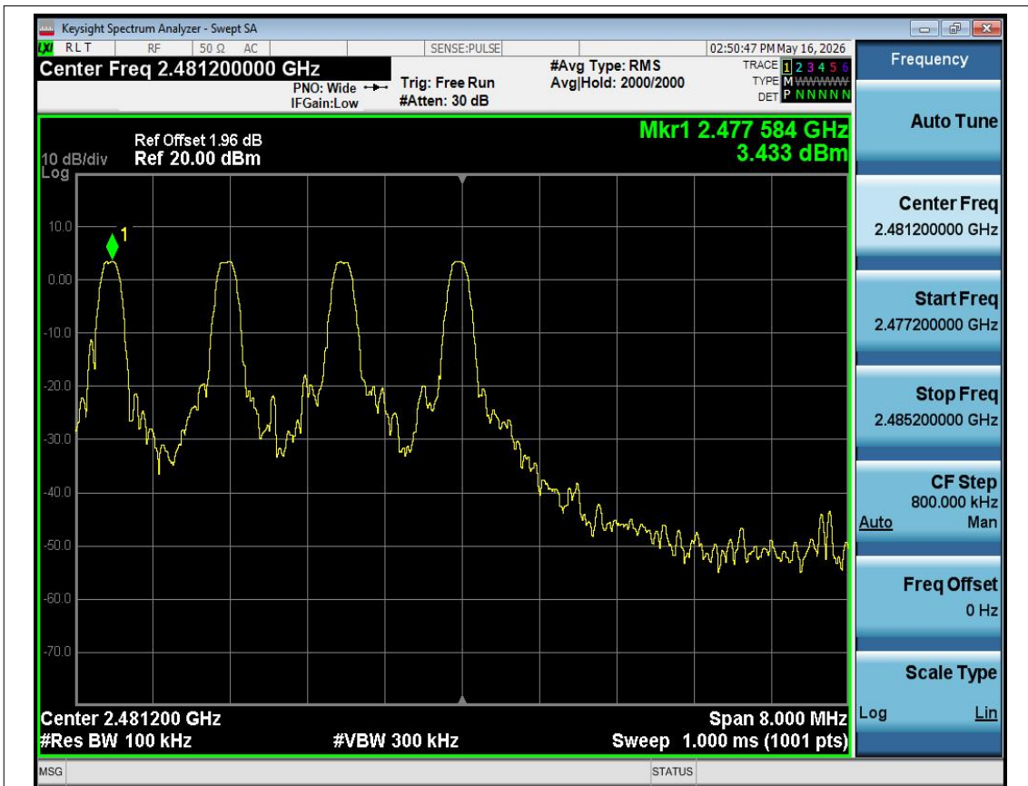
Band Edge(Hopping) NVNT 1-DH1 2481.2MHz Ant1 Hopping Ref
