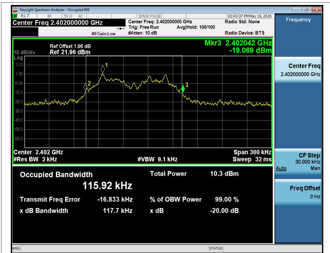
-20dB Bandwidth NVNT 1-DH1 2402MHz Ant1
