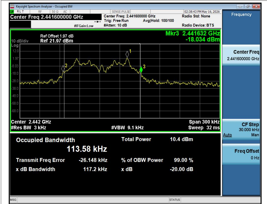
-20dB Bandwidth NVNT 1-DH1 2441.6MHz Ant1
